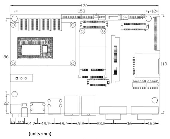
Figure 2.1: Mainboard Dimensions
