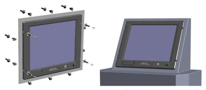
Figure 1.10: Panel Mounting of APC-3X20
