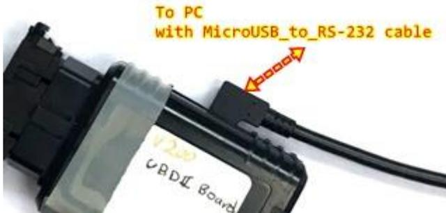
4. Make sure the COM port location of the USB to RS-232 cable recognized by PC (Win OS, Device Manage)
