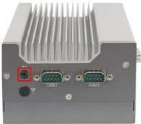
This connector supports Line-in and Line-out.
