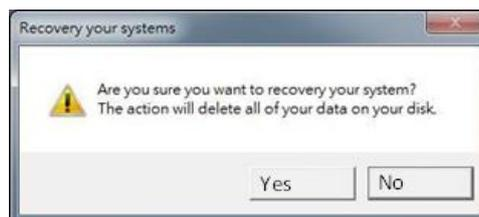
Wait the recovery process to complete. During the recovery process, a command prompt will show up to indicate the percent of recovery process complete. The system will restart automatically after recovery completed.
