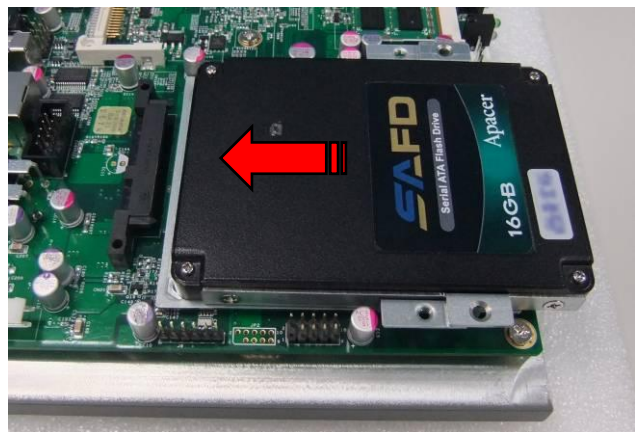
Fig. 8-4 Insert SSD into onboard SATA connector.
