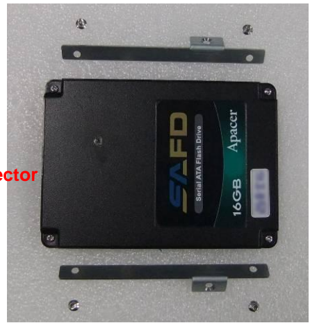
Fig. 8-2 Fasten brackets on SSD with four screws
