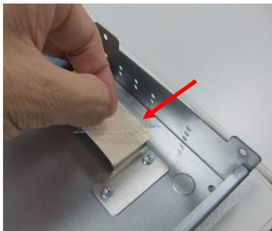
Fig. 7-1 Remove the film on thermal pad
