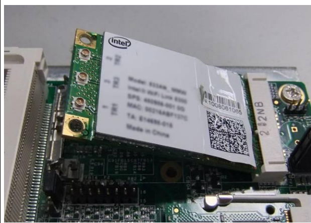
Fig. 9-1 Insert Mini PCI-e module (Supports USB signal only)
