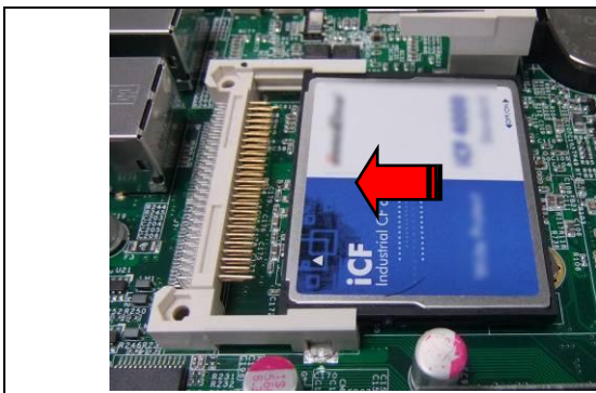
Fig. 6-1 Insert Compact Flash Card
