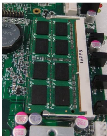
Fig. 7-3 Press down the memory module into socket
