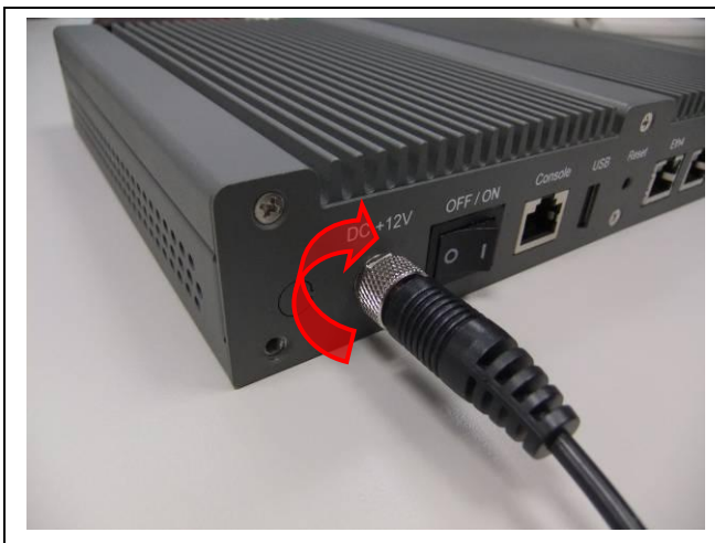
Fig. 10-1 Plug power connector into power jack
