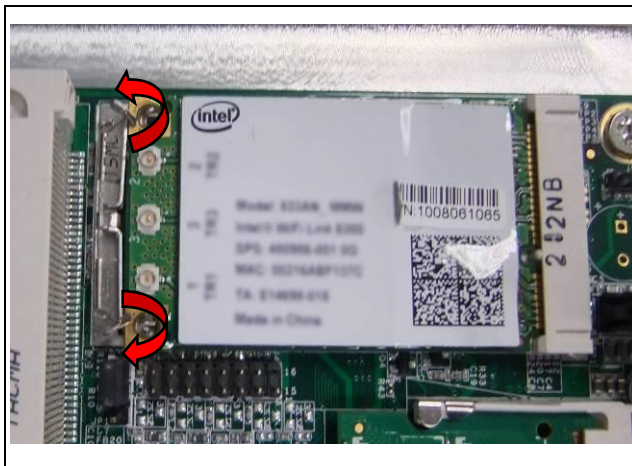
Fig. 9-3 Release two clips to remove module
