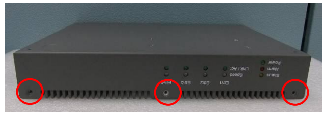
Fig. 5-2 Loosen three screws on front
