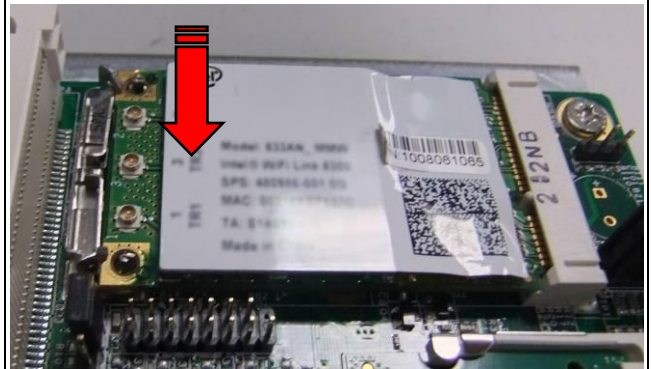
Fig. 9-2 Push down the module into socket
