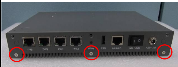
Fig. 5-1 Loosen three screws on back
