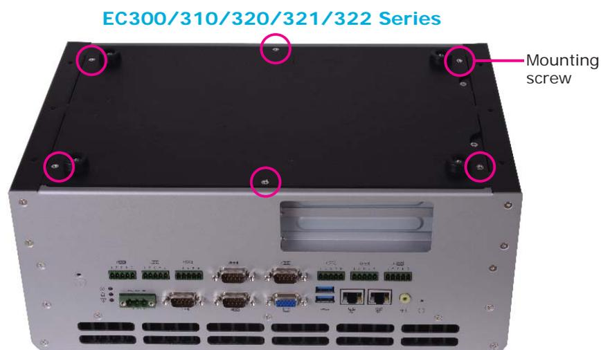
4. After removing the mounting screws, lift the cover up.
