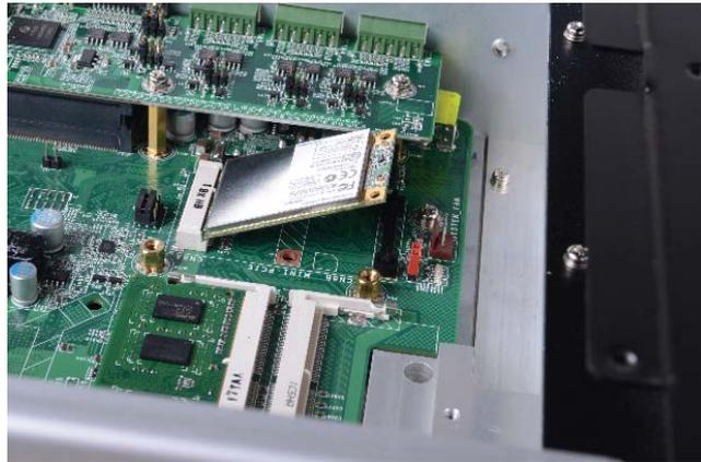
2. Push the Mini PCIe card down until the clips at each end of the latch lock into position. You will hear a distinctive “click”, indicating the card is correctly locked into position.
