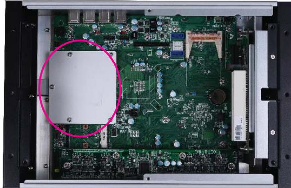
2. The 5 mounting screws on the protective plate is used to secure the plate. Remove these screws and then put them in a safe place for later use.
