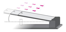
Step 2: Press the end of the card far from the socket down until against the stand-off.
