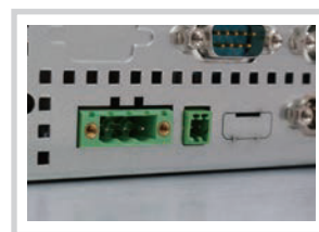
DC/AC Power Input, Support AT/ATX Mode
