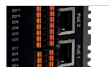
2 x PoE ports with intel GT210AT controller
