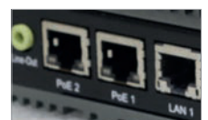
2 x PoE ports with Intel GT210AT Controller
