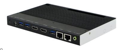
In addition, the SE-102-N supports extended operating temperatures of -40°F (-40°C) to +158°F (+70°C) and meets extreme system reliability requirements that allow for its use in a wide range of harsh outdoor environments. It features built-in hardware EDID (extended display identification data) simulation to prevent convergence issues caused by display/cable problems or failure to identify EDID.
