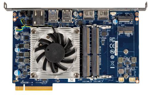
modules are ideal for low-power, basic signage applications. The Intel® SDM–L is designed for high-performance computing applications, with module dimensions of 175 mm  $\times$  100 mm (slightly less than 7"  $\times$  4") and a thickness of about 20 mm.
