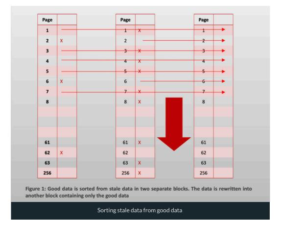
TRIM enables the SSD controller to skip invalid data instead of moving it. Naturally, this frees up a significant amount of resources and extends the lifespan of an SSD by reducing erase and write cycles on the SSD. TRIM tells the controller not to waste resources performing garbage collection on data in its logical block addresses (LBA) that has been designated invalid. See Figure 2.
