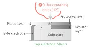
A High concentration of airborne sulfur-containing particles enters gaps in the resistor.
