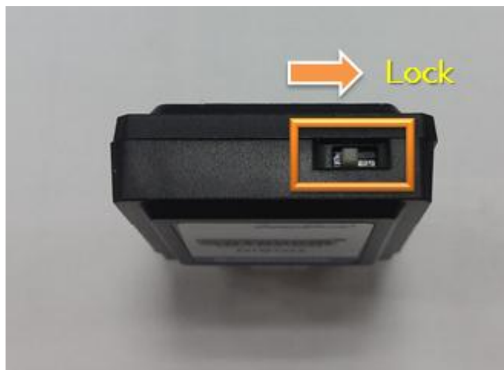
Figure 4: D150QV Write Protection Switch Direction
