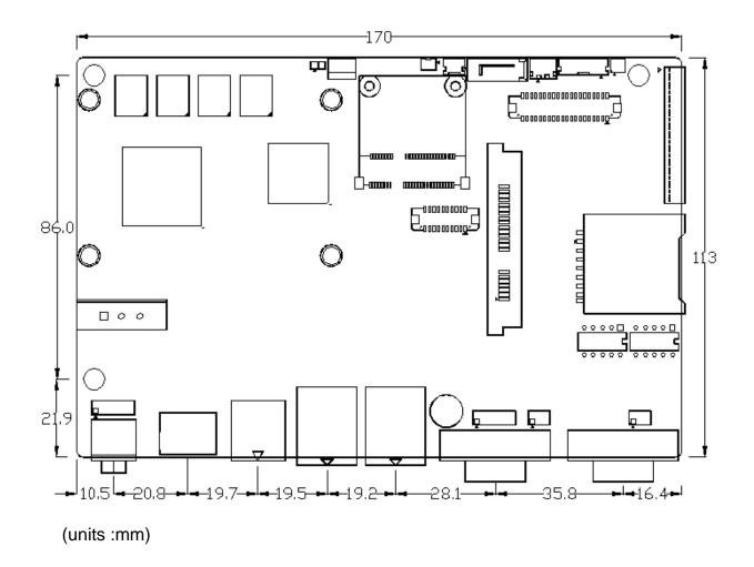
**Figure 2.1: Mainboard Dimensions**
