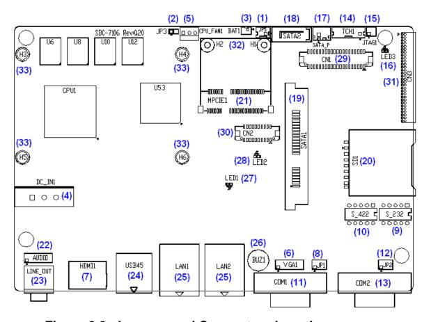
Figure 2.2: Jumpers and Connectors Location\_ Board Top
