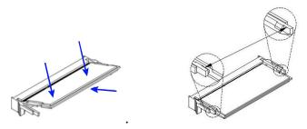
To remove the module, press the clips outwards with your thumb and index finger of both hands.
