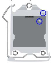
3. Carefully insert the CPU into the socket and push down the lever to secure the CPU.
