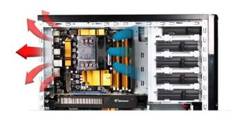
Excellent airflow design with compact heat sink dimension
