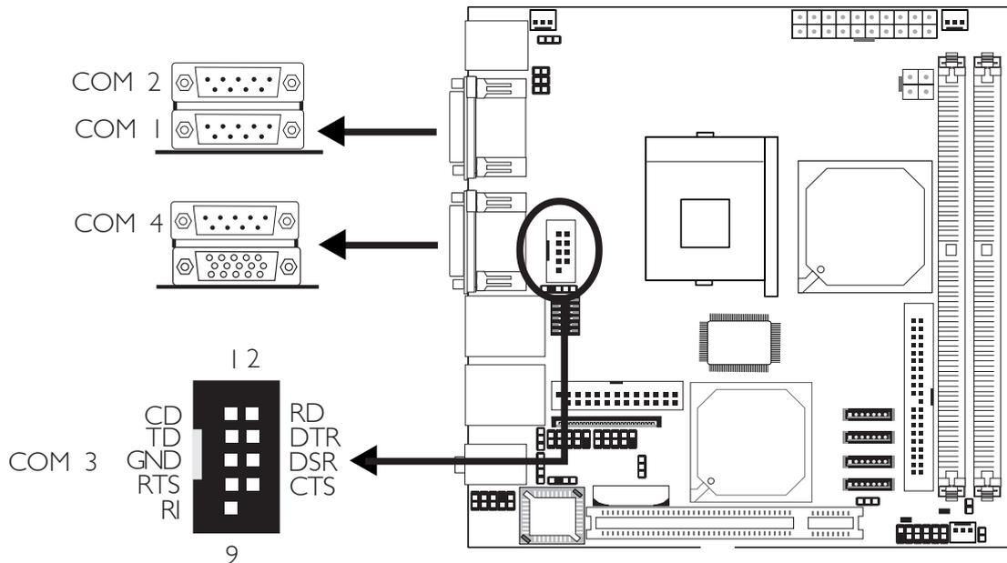
The system board is equipped with 3 onboard serial ports at locations CN5 (COM 1 and COM 2) and CN6 (COM 4). It is also equipped with a 9-pin connector for external COM 3 connection. These serial ports are RS-232 and/or RS-485 (COM 4 only) asynchronous communication ports with 16C550A-compatible UARTs that can be used with modems, serial printers, remote display terminals, and other serial devices.
