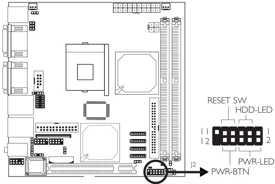
**HDD-LED - HDD LED**
