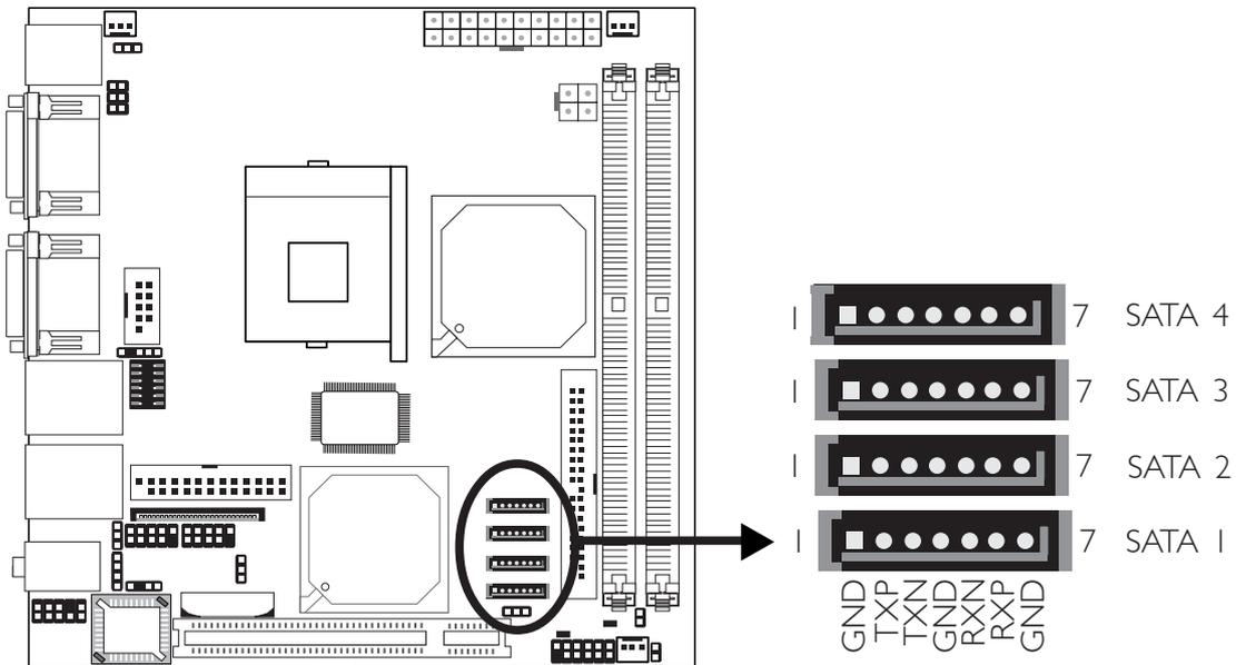
The system board is equipped with 4 Serial ATA connectors for connecting Serial ATA devices. Connect one end of the Serial ATA cable to the Serial ATA connector and the other end to your Serial ATA device.
