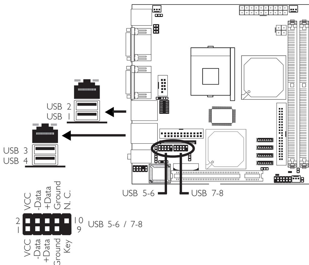
The system board supports 8 USB 2.0/1.1 ports. USB allows data exchange between your computer and a wide range of simultaneously accessible external Plug and Play peripherals.
