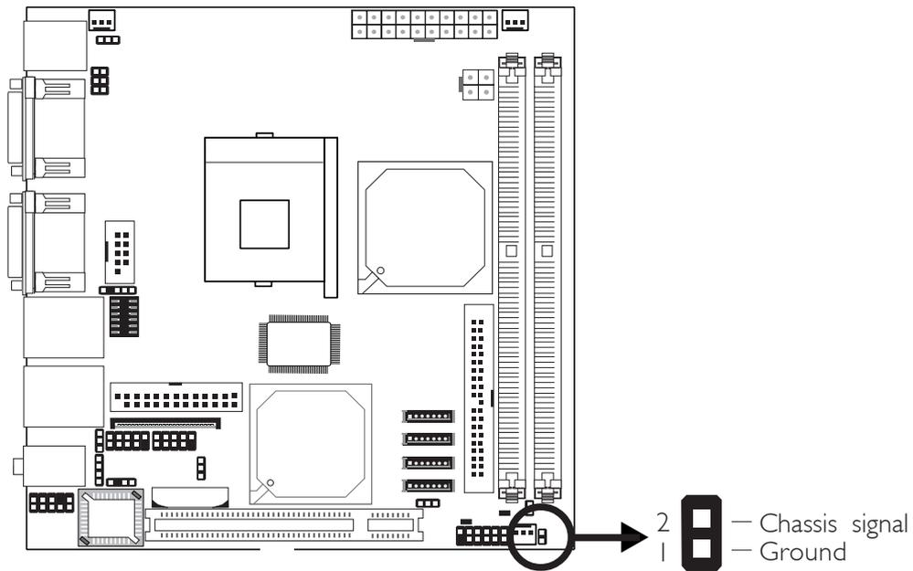
The system board supports the chassis intrusion detection function. Connect the chassis intrusion sensor cable from the chassis to the CASEOPEN1 connector. Whenever a chassis component has been removed, the sensor sends signal to CASEOPEN1 alerting you of a chassis intrusion event. To disable this function, place a jumper cap over CASEOPEN1.
