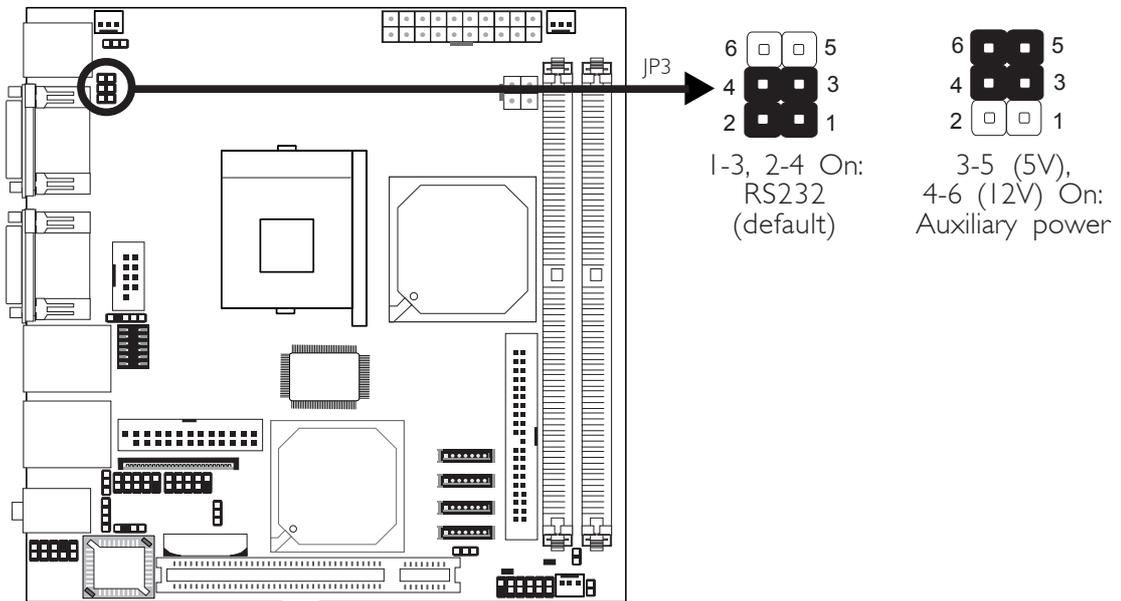
COM 2 is an RS-232 port. If the serial device connected to this port requires 5V/12V power from the system board, set JP3 pins 3-5 and 4-6 to On. Otherwise, leave this jumper's setting at 1-3, 2-4 On.
