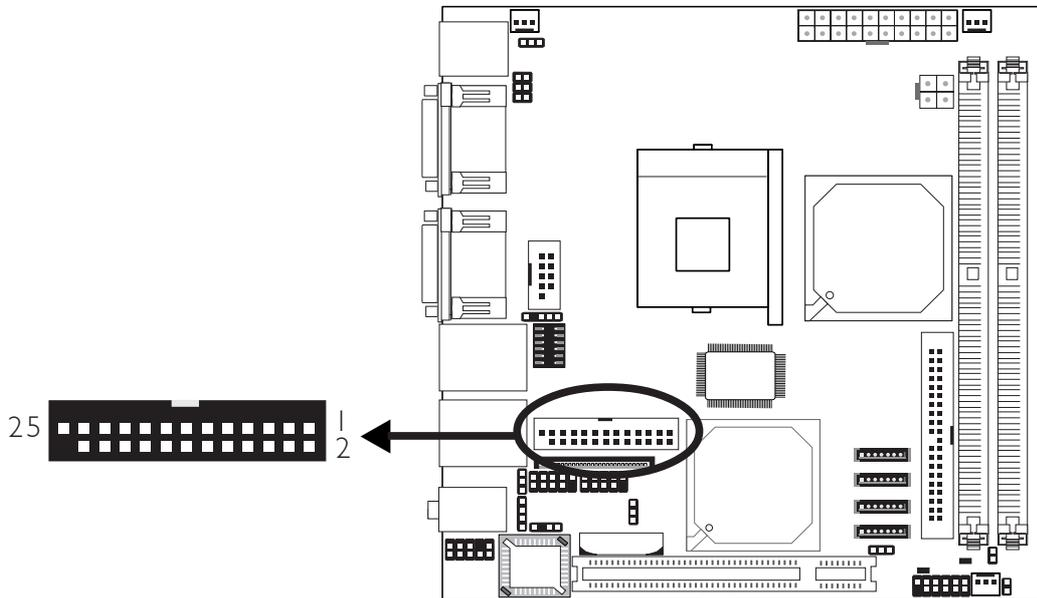
The 25-pin parallel connector is used for interfacing your PC to a parallel printer. It supports SPP, ECP and EPP.
