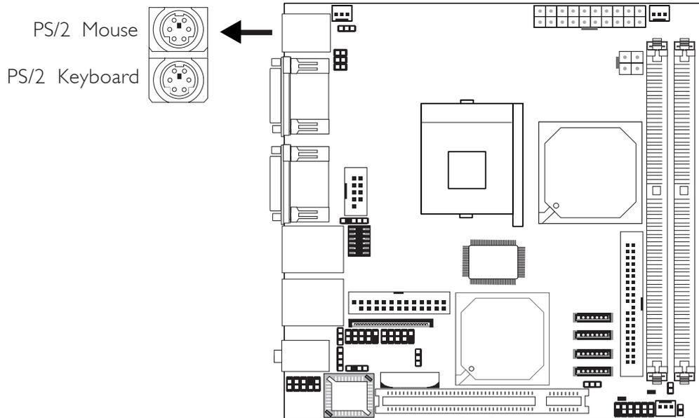
The system board is equipped with an onboard PS/2 mouse (Green) and PS/2 keyboard (Purple) ports - both at location CN1 of the system board. The PS/2 mouse port uses IRQ12. If a mouse is not connected to this port, the system will reserve IRQ12 for other expansion cards.
