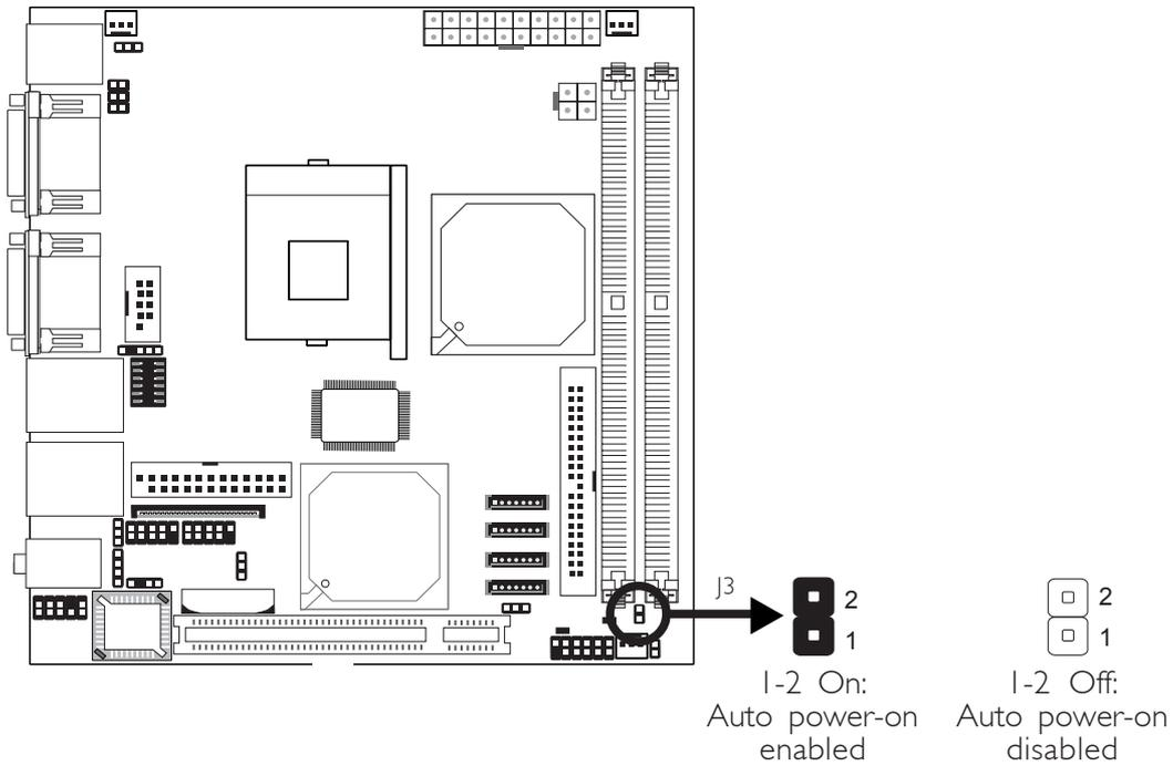
If you want the system to automatically power-on once AC power comes in, set J3 pins 1 and 2 to On.
