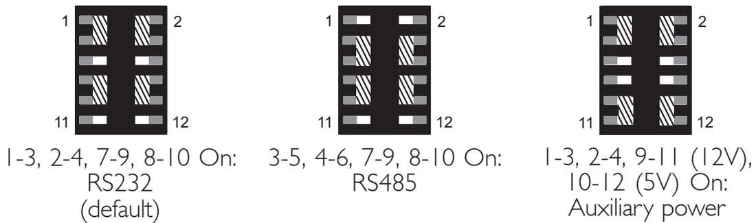
JP4 is used to set COM 4 to RS-232 or RS-485. If the serial device connected to this port requires 5V/12V power from the system board, set JP4 pins 1-3, 2-4, 9-11 and 10-12 to On. This setting automatically sets COM 4 at RS-232.
