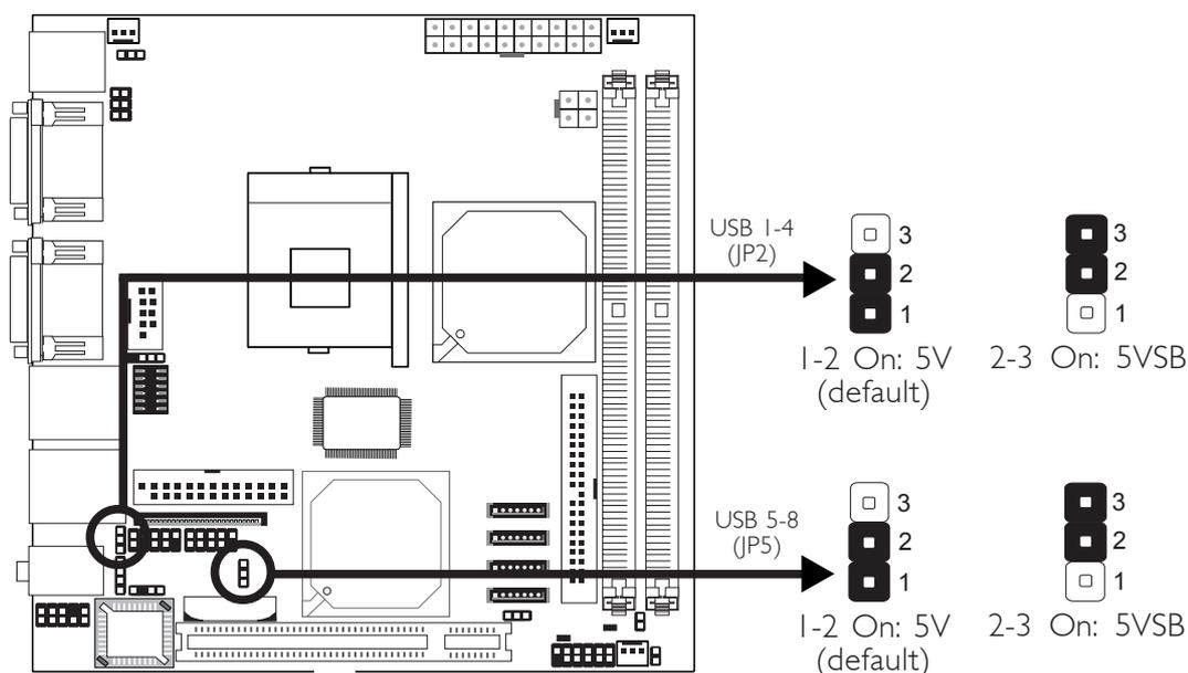
JP2 and JP5 are used to select the power of the USB ports. Selecting 5VSB will allow you to use the USB keyboard or USB mouse to wake up the system.
