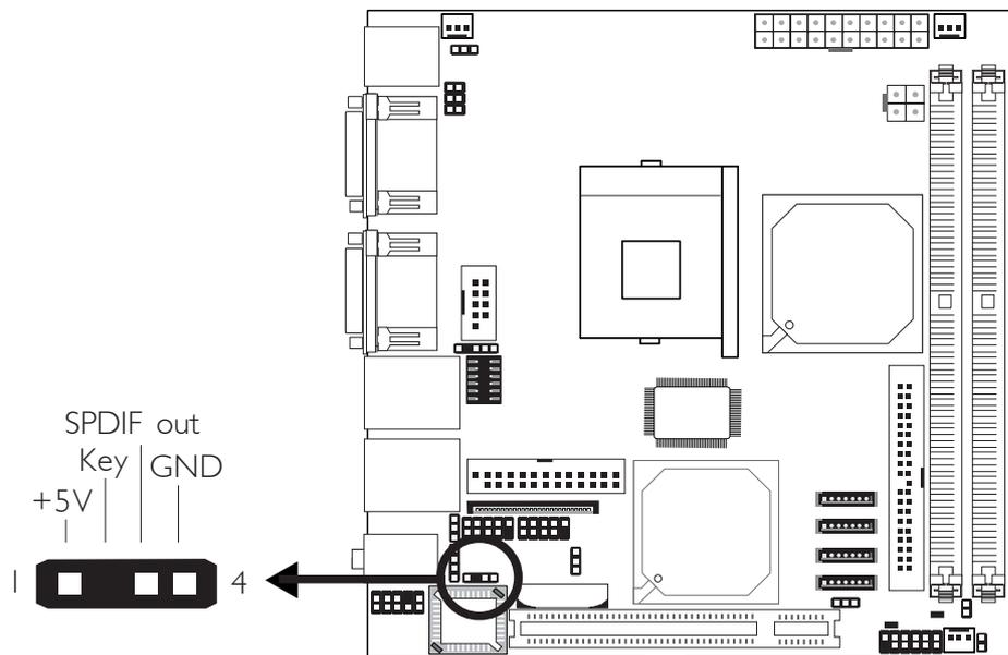
The system board is equipped with a S/PDIF-out connector. One card-edge bracket, mounted with S/PDIF-out port, may be provided with the system board. Install the card-edge bracket to the system chassis then connect the audio cable connector to the SPDIF I connector. Make sure pin 1 of the audio cable connector is aligned with pin 1 of SPDIF I.
