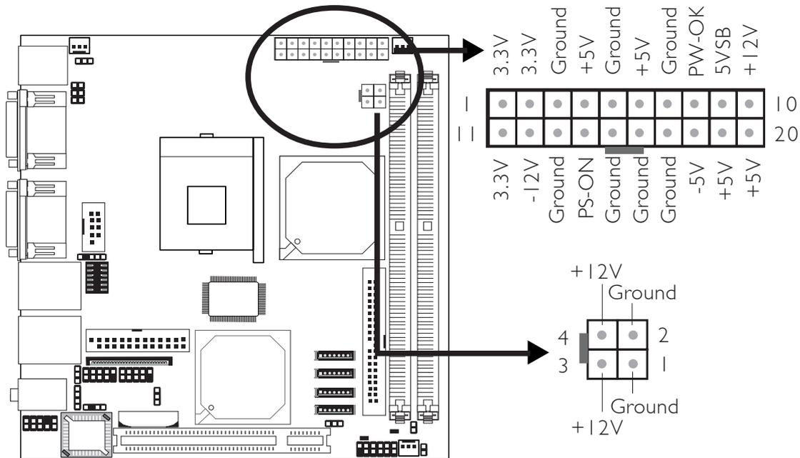
We recommend that you use a power supply that complies with the ATX12V Power Supply Design Guide Version 1.1. An ATX12V power supply has a standard 20-pin ATX main power connector and a 4-pin +12V power connector that must be inserted onto P1 and P2 connectors respectively.
