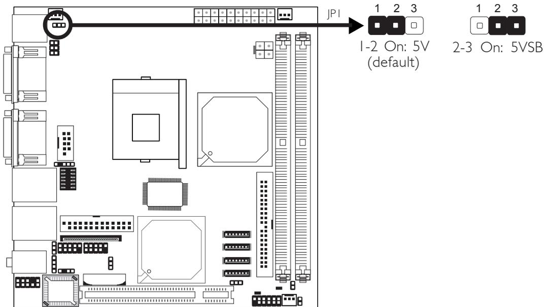
JPI is used to select the power of the PS/2 keyboard/mouse port. Selecting 5VSB will allow you to use the PS/2 keyboard or PS/2 mouse to wake up the system.
