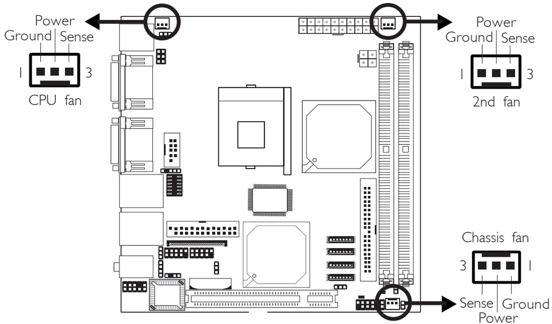
Connect the CPU fan's cable connector to the CPU fan connector on the system board. The 2nd fan and chassis fan connectors are used to connect additional cooling fans. The cooling fans will provide adequate airflow throughout the chassis to prevent overheating the CPU and system board components.
