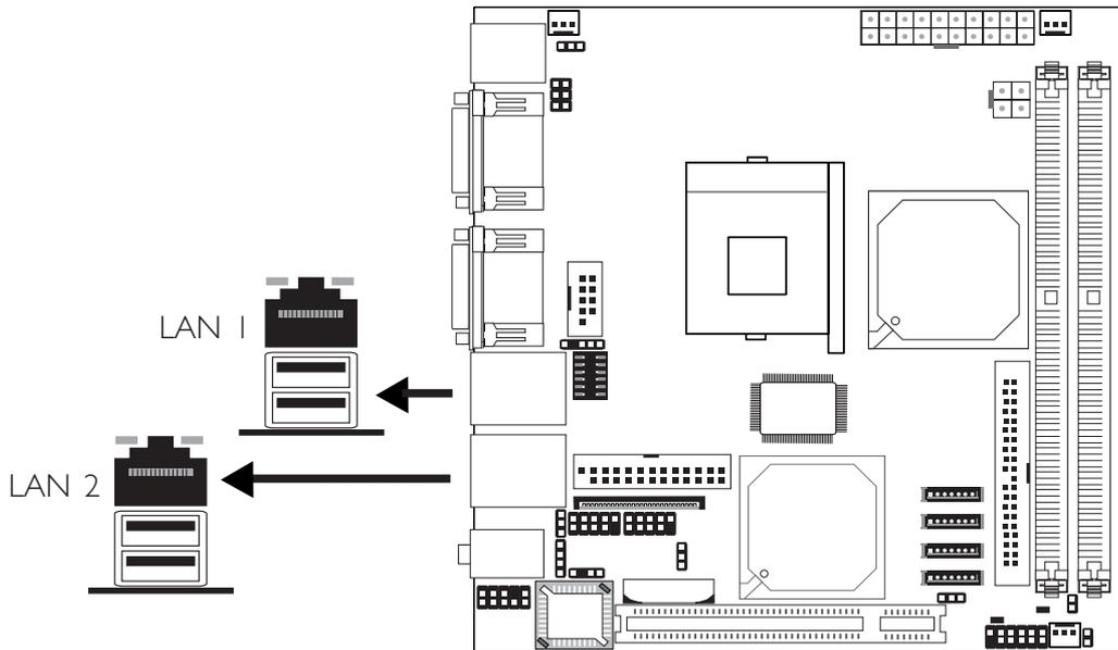
The system board is equipped with two onboard RJ45 Gigabit LAN ports at locations CN4 (LAN 1) and CN3 (LAN 2). These ports allow the system board to connect to a local area network by means of a network hub.
