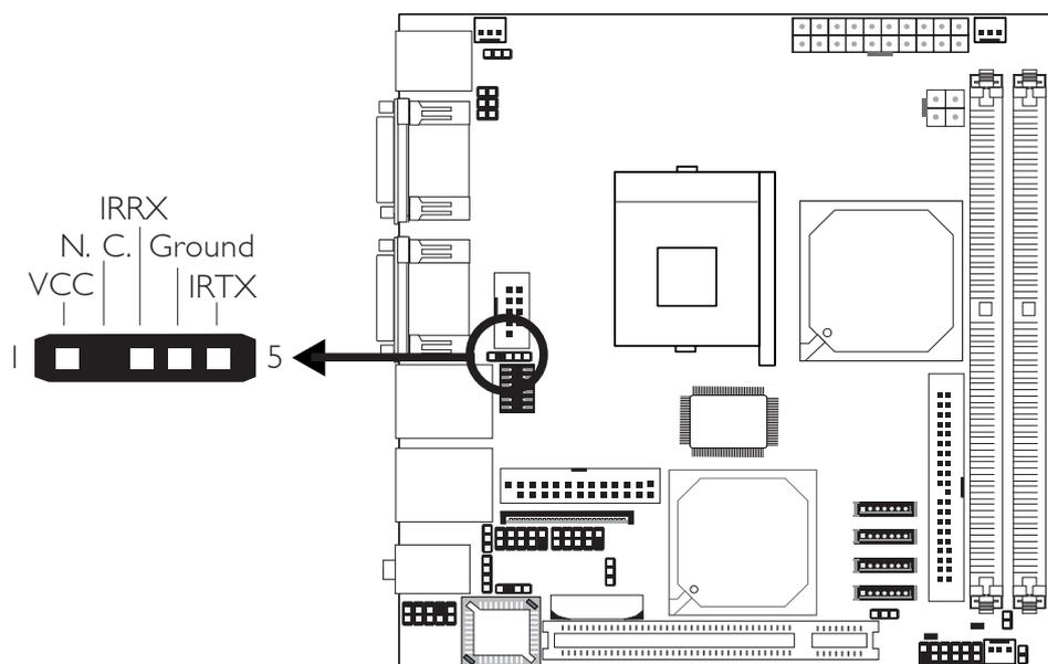
Connect your IrDA cable to the IrDA connector on the system board.
