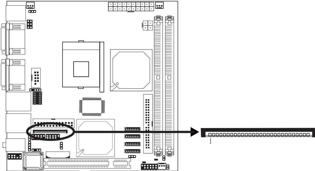
The system board is equipped with a 26-pin FPC type floppy disk drive connector. Only connect a 1.44MB slim-type floppy disk drive. Floppy drives other than the one mentioned above are optional. Refer to the next page for the pin function of this connector:
