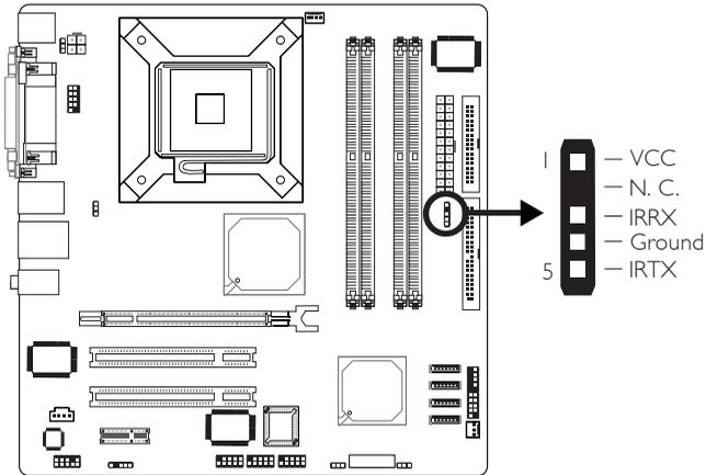
Connect the cable connector from your IR module to the IR connector (J13).
