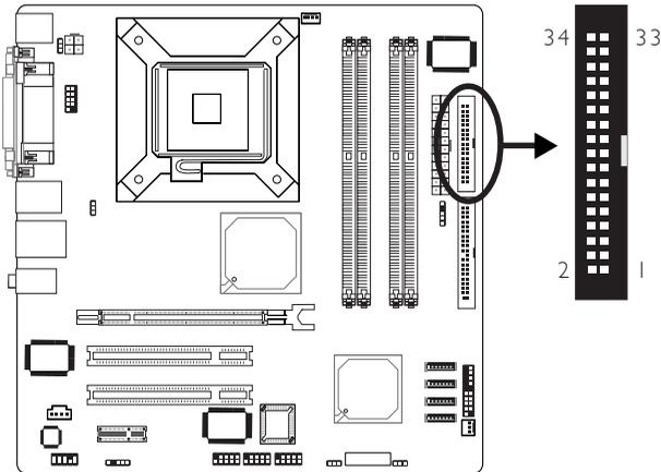
The system board is equipped with a shrouded floppy disk drive connector that supports two standard floppy disk drives. To prevent improper floppy cable installation, the shrouded floppy disk header has a keying mechanism. The 34-pin connector on the floppy cable can be placed into the header only if pin 1 of the connector is aligned with pin 1 of the header.
