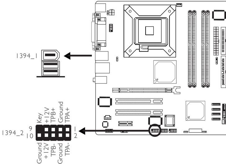
The system board is equipped with an onboard IEEE 1394 port at location CN1 (IEEE 1394\_1).
