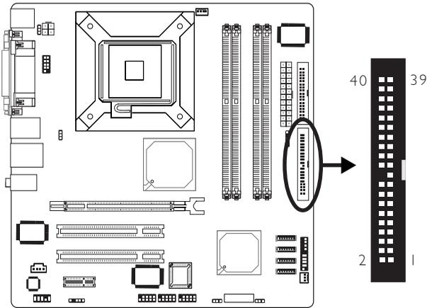
The system board is equipped with a shrouded PCI IDE header that will interface two Enhanced IDE (Integrated Drive Electronics) disk drives. To prevent improper IDE cable installation, the shrouded PCI IDE header has a keying mechanism. The 40-pin connector on the IDE cable can be placed into the header only if pin 1 of the connector is aligned with pin 1 of the header.
