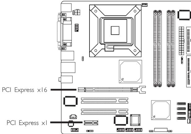
The system board is equipped with one PCI Express x16 and one PCI Express x1 slots.
