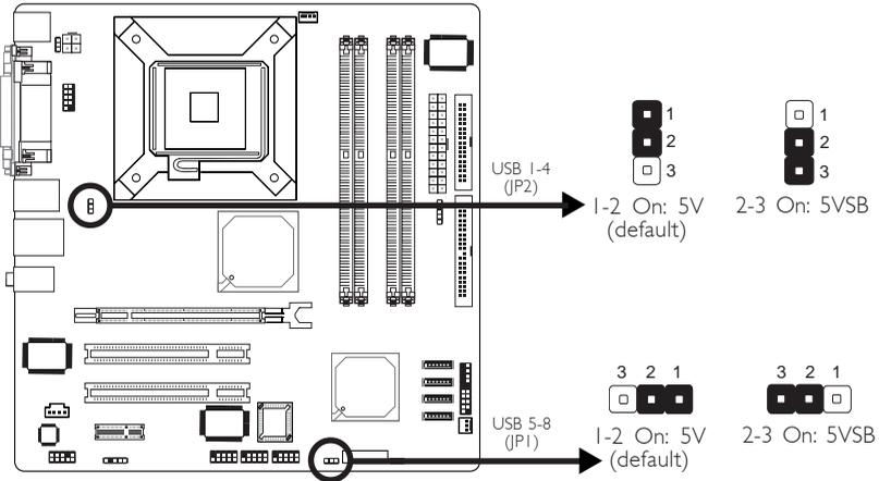
JP1 and JP2 are used to select the power of the USB ports. Selecting 5VSB will allow you to use the USB keyboard or USB mouse to wake up the system.
