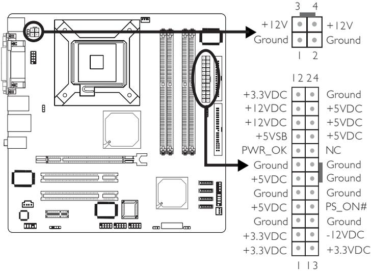
We recommend that you use a power supply that complies with the ATX12V Power Supply Design Guide Version 1.1. An ATX12V power supply has a standard 24-pin ATX main power connector and a 4-pin +12V power connector that must be inserted onto CN8 and CN9 connectors respectively.
