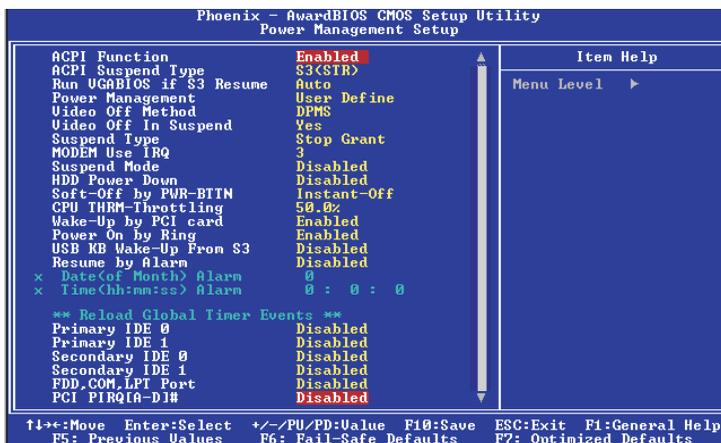
The screen above list all the fields available in the Power Management Setup submenu, for ease of reference in this manual. In the actual CMOS setup, you have to use the scroll bar to view the fields. The settings on the screen are for reference only. Your version may not be identical to this one.
