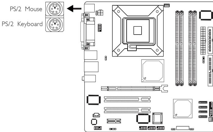
The system board is equipped with an onboard PS/2 mouse (Green) and PS/2 keyboard (Purple) ports - both at location CN7 of the system board. The PS/2 mouse port uses IRQ12. If a mouse is not connected to this port, the system will reserve IRQ12 for other expansion cards.
