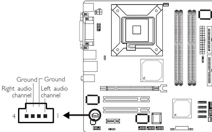
The CD-in (J6) connector is used to receive audio from a CD-ROM drive, TV tuner or MPEG card.
