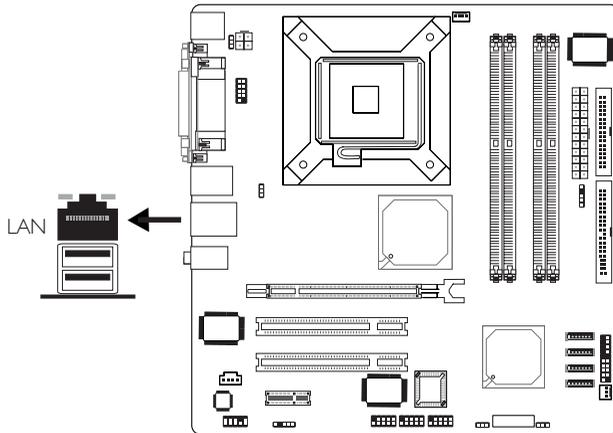
The RJ45 LAN port is at location CN2 of the system board. LAN allows the system board to connect to a local area network by means of a network hub.
