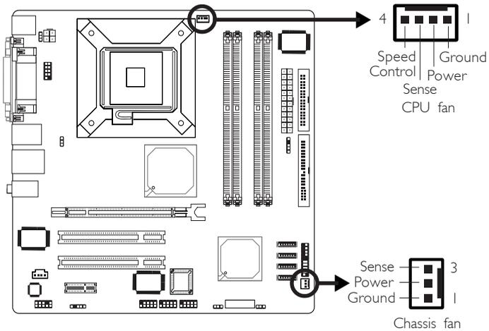
Connect the CPU fan's cable connector to the CPU fan connector (J8) on the system board. The chassis fan connector (J10) is used to connect an additional cooling fan. The cooling fan will provide adequate airflow throughout the chassis to prevent overheating the CPU and system board components.
