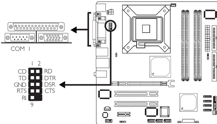
The system board is equipped with an onboard serial port (Teal/Turquoise) at location CN5 for COM 1. It is also equipped with a 9-pin connector at location J9 for COM 2. The serial ports are RS-232C asynchronous communication port with 16C550A-compatible UARTs that can be used with a modem, serial printer, remote display terminal or other serial devices.
