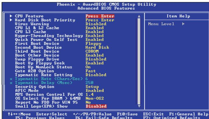
The screen above list all the fields available in the Advanced BIOS Features submenu, for ease of reference in this manual. In the actual CMOS setup, you have to use the scroll bar to view the fields. The settings on the screen are for reference only. Your version may not be identical to this one.
