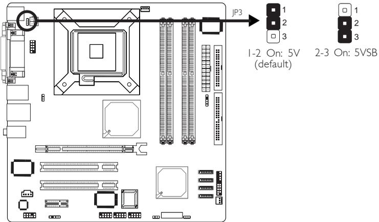
JP3 is used to select the power of the PS/2 keyboard/mouse port. Selecting 5VSB will allow you to use the PS/2 keyboard or PS/2 mouse to wake up the system.
