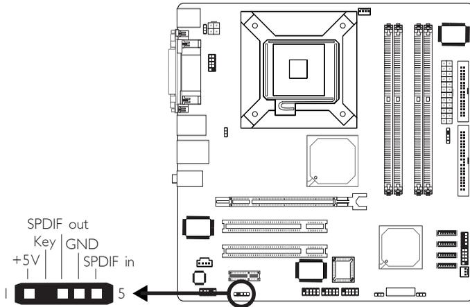
The system board is equipped with a S/PDIF connector. One card-edge bracket, mounted with S/PDIF ports, may be provided with the system board. Install the card-edge bracket to the system chassis then connect the audio cable connector to J5. Make sure pin 1 of the audio cable connector is aligned with pin 1 of J5.
