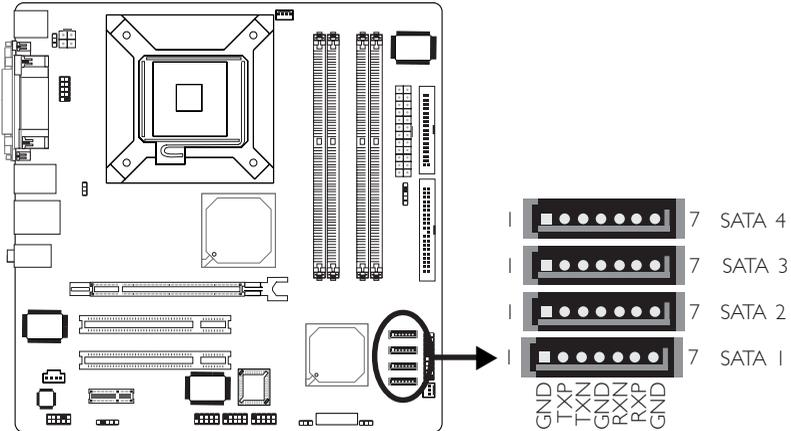
The system board is equipped with four Serial ATA connectors for connecting Serial ATA devices. Connect one end of the Serial ATA cable to J15 (SATA 1), J16 (SATA 2), J17 (SATA 3) or J18 (SATA 4) and the other end to your Serial ATA device.
