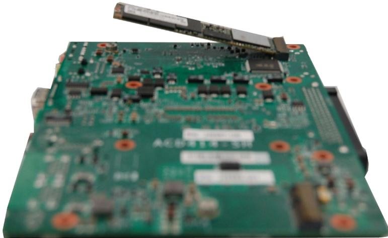
3. Secure the card to the riser screw on the board using the screw shipped with the M.2 module.
