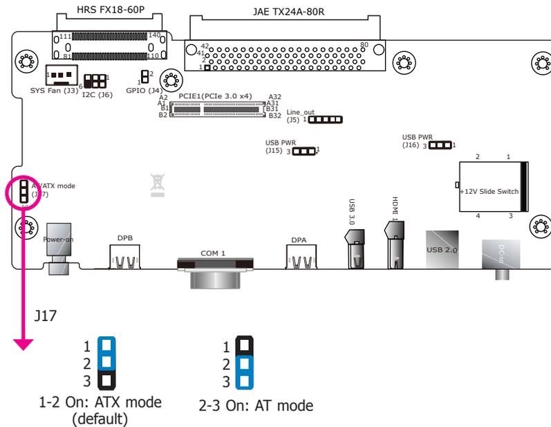
J17 is used to select the power-on mode: AT or ATX (default). The Docking Board is equipped with a hard switch to provide AT power scheme. With the AT mode, you need to manually turn off the system with the power switch; whereas in the ATX mode, the system can be powered off using the shut-down function provided by the OS.
