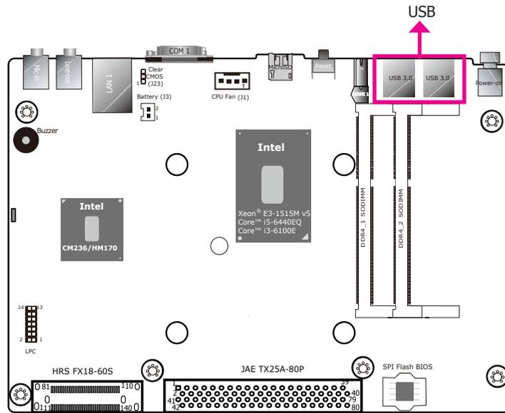
The OPS100-SH is equipped with four USB 3.0 port. USB devices allow data exchange between your computer and a wide range of simultaneously accessible external Plug and Play peripherals.
