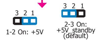
J15 and J16 are used to select the power for the Docking Board's USB port 3.0 and USB ports 2.0 respectively. Selecting +5V\_standby will allow you to use USB devices to wake up the system.
