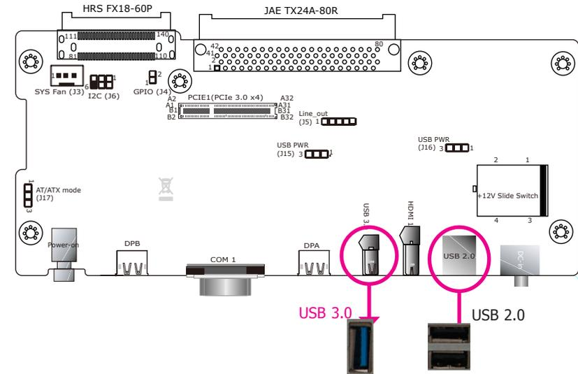
The Docking Board is equipped with one USB 3.0 and two USB 2.0 ports. The USB 3.0 can transfer data up to 5 Gbps whereas the USB 2.0 can transfer data up to 480Mbps.
