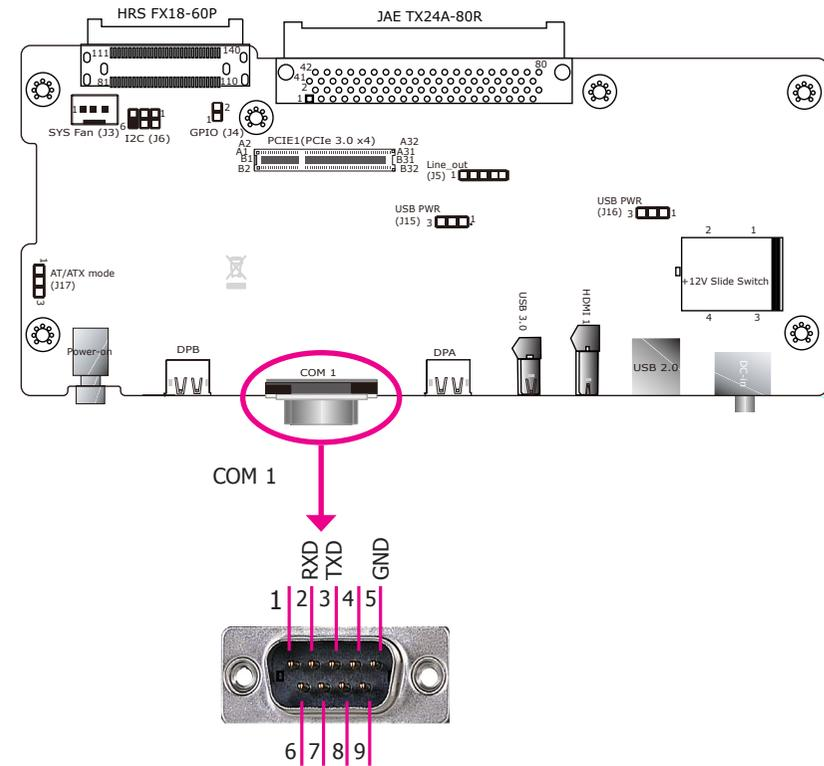
Unlike a normal 9-pin RS232 serial port, this COM port only provides RX and TX communication links.
