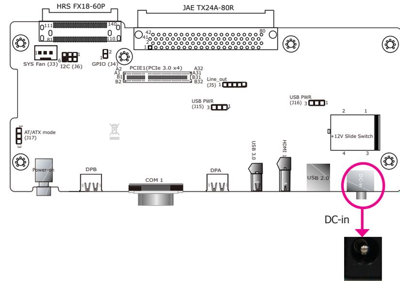
Connect a DC power cord to this DC-in jack. Using a voltage more than the recommended range may fail to boot the system or damage the system board.
