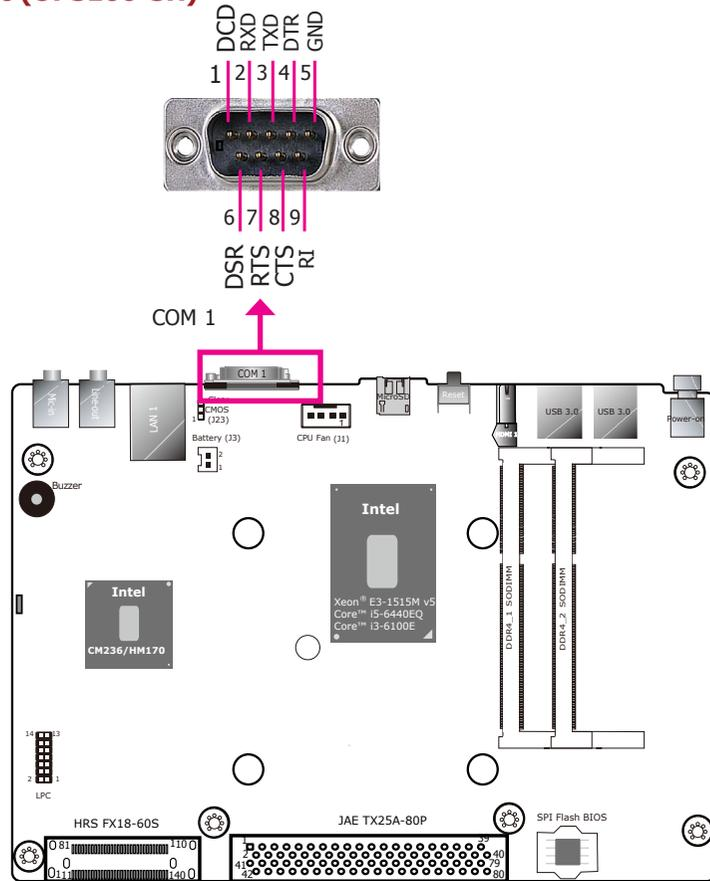
This COM port is an RS232 port and provides 9-pin serial communication.
