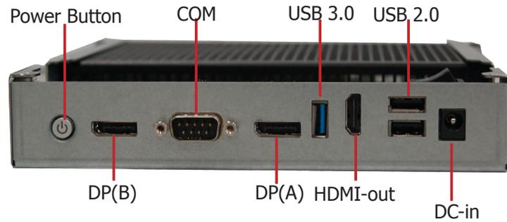
The Docking Board provides these additional I/O ports:
