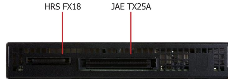
The rear panel I/O consists of the following ports:
