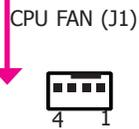
The fan connector is used to connect the cooling fan of a CPU heatsink.
