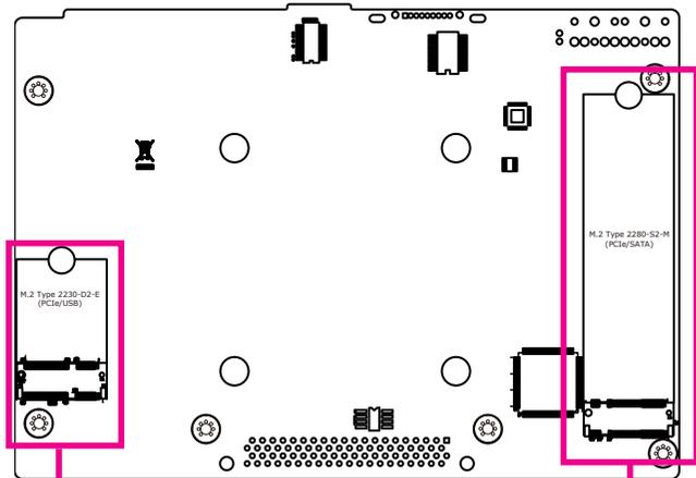
M.2 Type 2230 connector (for both PCI Express and USB 2.0 interfaces)
