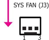
The fan connector is used to connect a cooling fan for the system.
