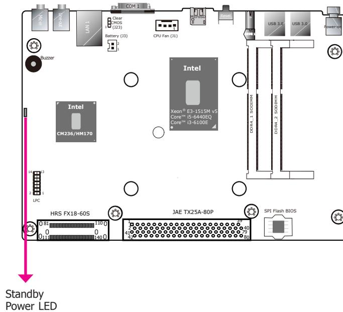
This LED will be lit when the system is in the standby mode. It indicates that there is power on the system board. Power off the system and then unplug the power cord prior to installing any devices. Failure to do so will cause severe damage to the motherboard and components.
