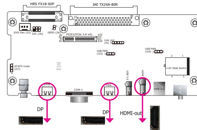
Using the Docking Board, the system supports triple display with the following output interfaces:
