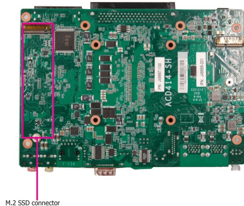
2. Insert the M.2 module into the connector.
