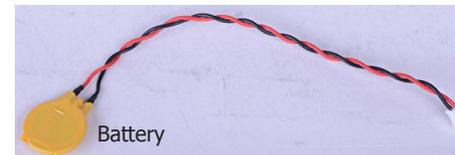
The lithium ion battery powers the real-time clock and CMOS memory. It is an auxiliary source of power when the main power is shut off.
