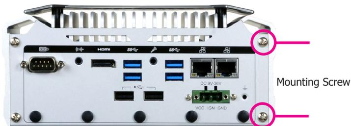
2. Align the mounting holes on the system and the mounting holes on the bracket, and then use the screws removed in step 1 to secure the bracket in place.
