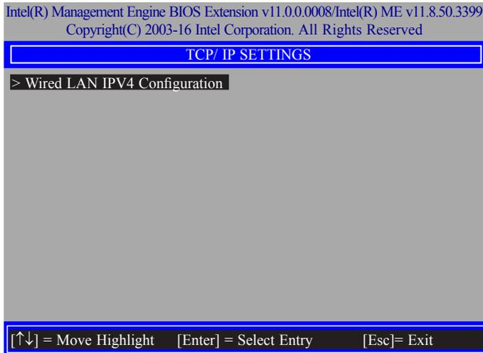
27. In the "TCP/IP Settings" menu, select "Wired LAN IPV4 Configuration" and then press "Enter".
