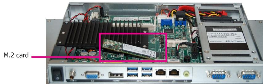
4. Push down on the other end of the M.2 card and secure the card on the mainboard with the provided mounting screw.
