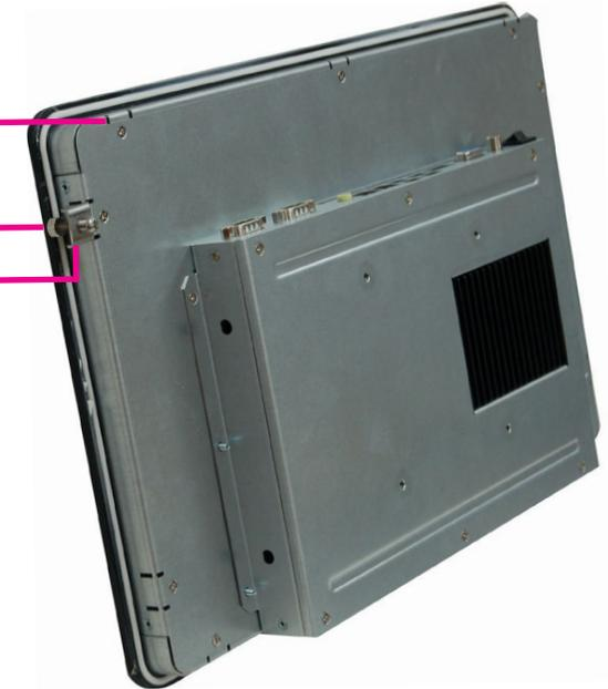
5. The first and second clamps must be positioned and secured diagonally prior to mounting the rest of the clamps. Tighten the clamp's screw using an electric screwdriver by pressing the white plastic cap onto the back of the panel. The illustration below shows that all clamps are properly mounted.
