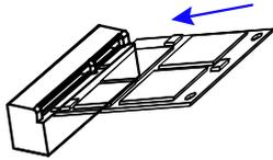
3. Push the mini-PCle card down and fix it with the an M2 screw. (Fix the M.2 network card with an M3 screw.)
