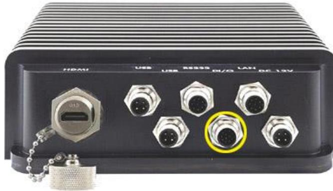
Digital I/O Cable: M12 to open wire
