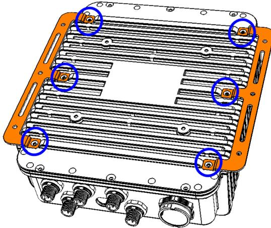
2. Prepare 4 screws (M3) to install the device on the wall, as shown.
