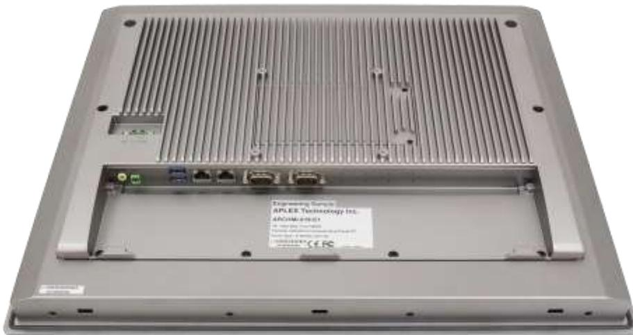
**Figure 1.28: Rear View of ARCHMI-819(P)H**
