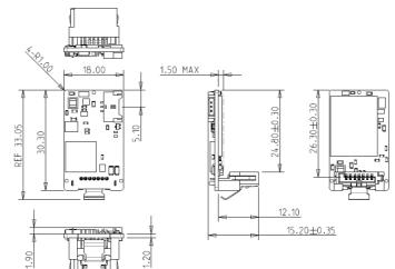
TOLERANCE: ±0.20mm UNIT: mm
