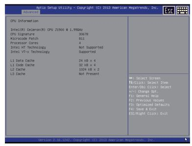
CPU Type/Signature/Microcode Path/Processor Cores/64-bit/Intel HT Technology/ Intel VT-x Technology
