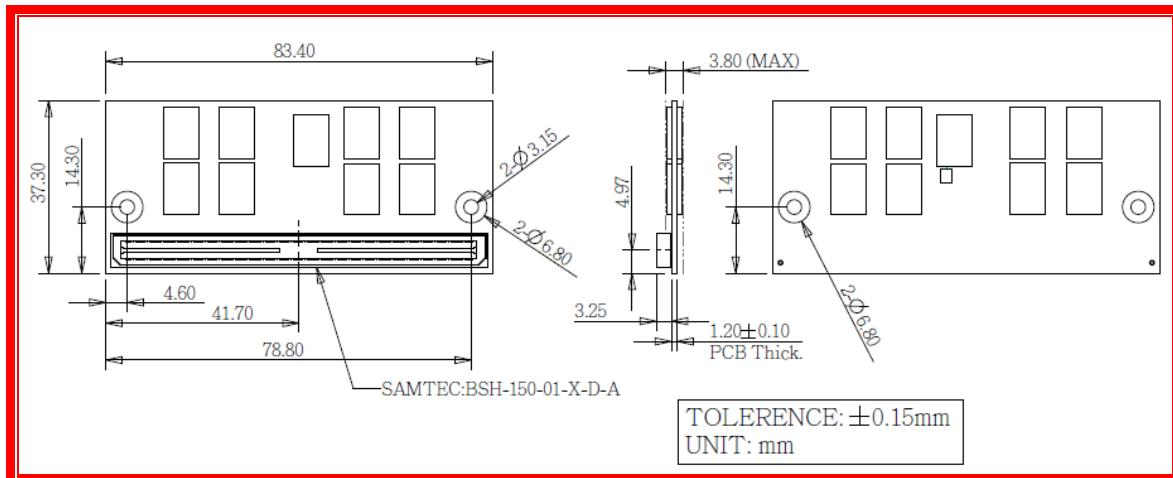
Note: All dimensions are in millimeters and should be kept within a tolerance of  $\pm 0.15$ , unless otherwise specified.
