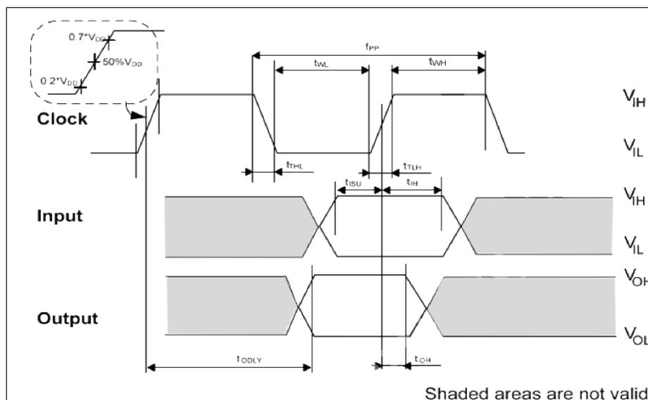
Figure 6: Timing diagram data input/output referenced to clock
