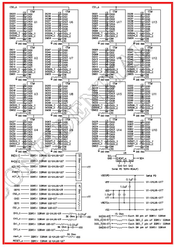
Note: 1. The ZQ ball on each DDR4 component is connected to an external 240 $\Omega$  ±1% resistor that is tied to ground. It is used for the calibration of the component's ODT and output driver.
