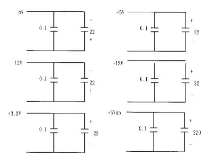
0.1uf is ceramic, the other is tantalum. Noise bandwidth is from DC to 20Mhz
