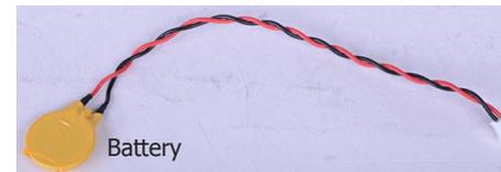
The lithium ion battery powers the real-time clock and CMOS memory. It is an auxiliary source of power when the main power is shut off.
