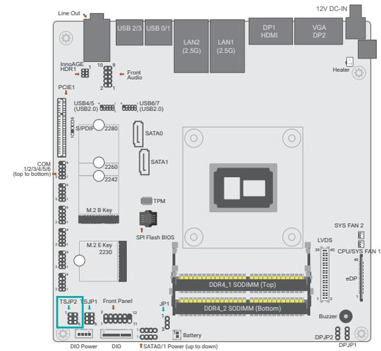
This jumper is to determine the COM2 Power.
