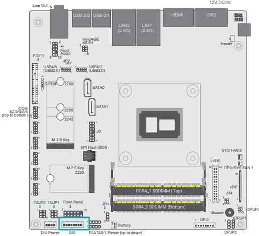
The 8-bit Digital I/O connector provides powering-on function to external devices that are connected to these connectors. The pin functions of the 8-bit digital I/O connector are listed below.
