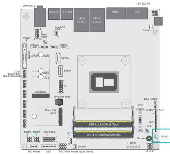
This jumper is to determine the dimming of panel backlight.
