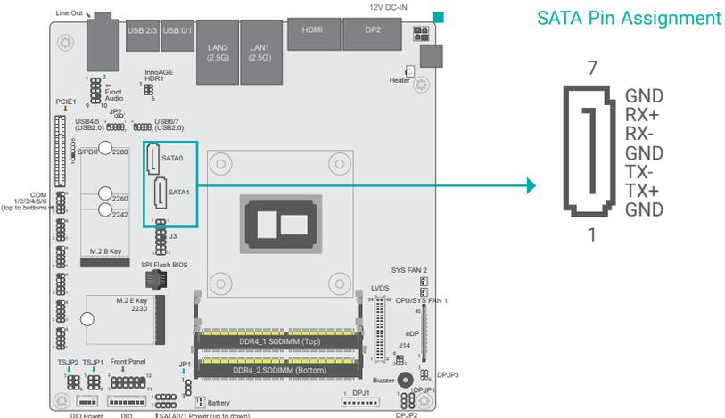
The Serial ATA (SATA) connectors are used to connect the Serial ATA device. SATA 3.0 is supported by the 2 SATA ports and provides data rate up to 6Gb/s. Connect one end of the Serial ATA cable to a SATA connector and the other end to your Serial ATA device.
