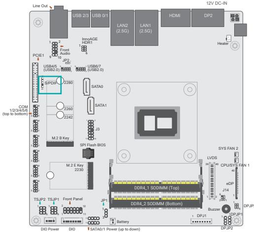
The S/PDIF connector is used to connect an external S/PDIF port. Your S/PDIF port may be mounted on a card-edge bracket. Install the card-edge bracket to an available slot at the rear of the system chassis then connect the audio cable to the S/PDIF connector. Make sure pin 1 of the audio cable is aligned with pin 1 of the S/PDIF connector.
