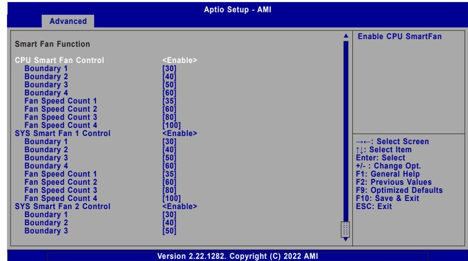
Smart Fan is a fan speed moderation strategy dependent on the current system temperature. When the system temperature goes higher than the Boundary setting, the fan speed will be turned up to the setting of the Fan Speed Count that bears the same index as the Boundary field.
