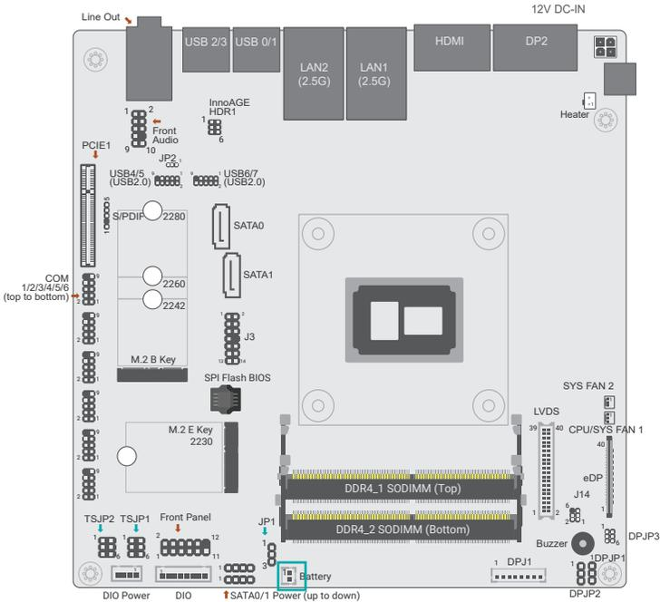
The lithium ion battery addendum supplies power to the real-time clock and CMOS memory as an auxiliary source of power when the main power is shut off. Plug the battery cable into the header.
