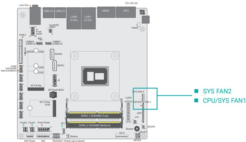
These fan connectors are used to connect cooling fans. The cooling fans will provide adequate airflow throughout the chassis to prevent overheating the CPU and system board components.
