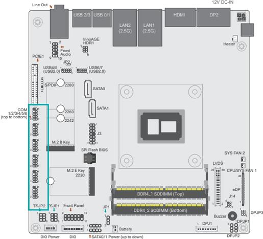
**Connecting External Serial Ports**
