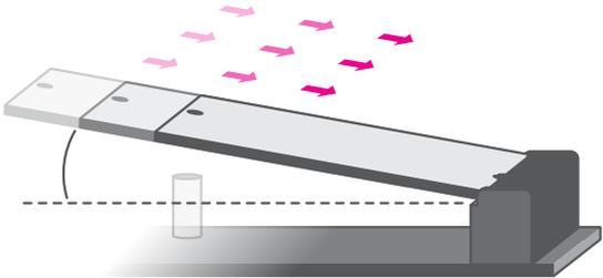
Step 1: Insert the card into the socket at an angle while making sure the notch and key are perfectly aligned.
