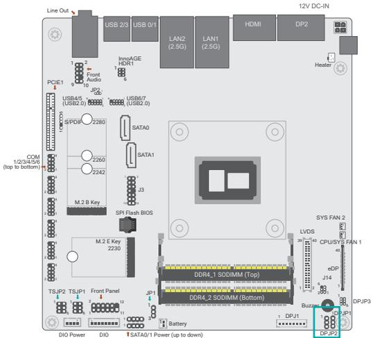
This jumper is to determine the power of panel inverter.
