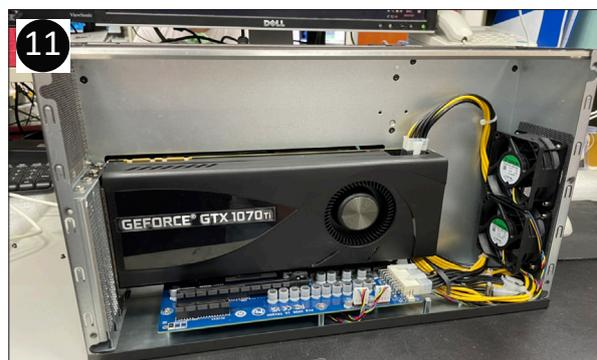
NOTE 1 : To connect 1 or 2 power cables on the graphic cards is depends on different graphic card spec.
