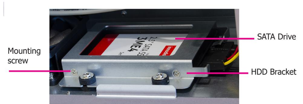
2. Place the HDD bracket with the installed SATA drives back into the chassis and use the provided mounting screws to attach the HDD bracket to the drive bay. Use the provided mounting screws to attach the HDD bracket to the drive bay.
