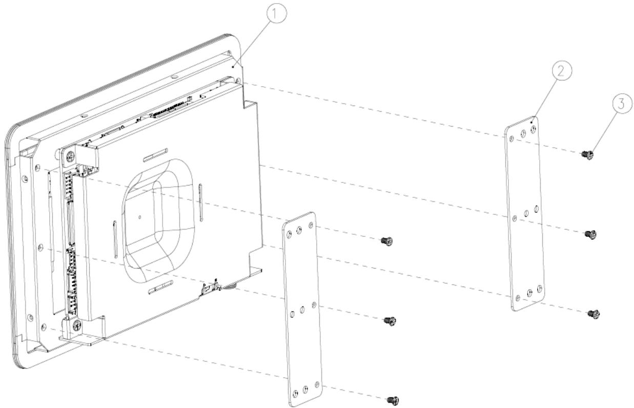
**Step1.** Locate brackets on both sides, matching the holes on the monitor.
