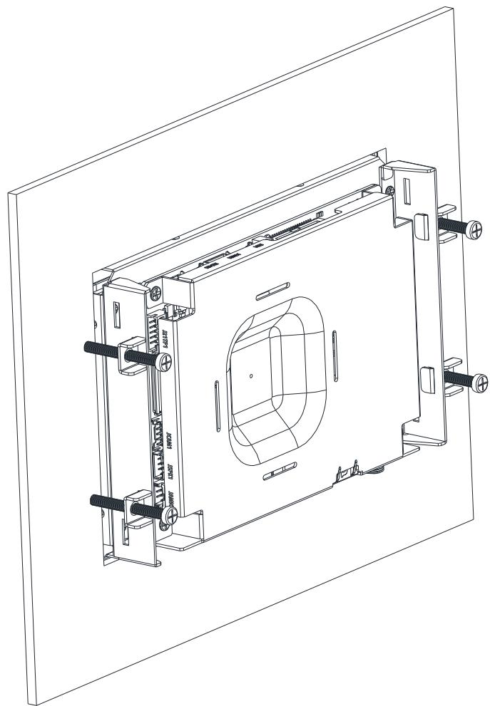
**Step4.** Insert and fasten 4 Panel mount screws to secure the module.
