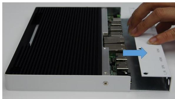
2. Push the mSATA module into the slot. Screw two screws to secure the module in the slot.
