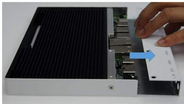
2. Push the WIFI module into the slot. Screw two screws to secure the module in the slot.
