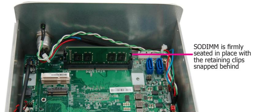
To remove a SODIMM, gently spread the retaining clips at each end of the SODIMM socket. The SODIMM should pop out of the socket. Lift the SODIMM away from the socket on the mainboard.
