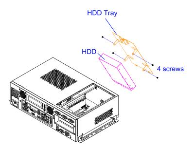
3. Put the tray back and tighten the screw mentioned in Step 1 to secure the HDD tray.
