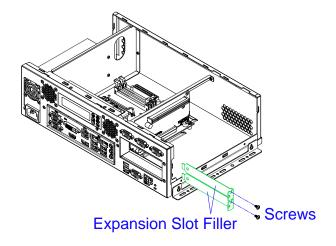
3. Install your PCIe (x16) expansion card and fix the card by tightening the screw mentioned above.
