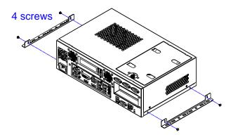
2. Then prepare at least four screws (M3, 6 mm) to mount the device on wall .
