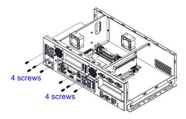
After installation, tighten 6 screws mentioned in Step 1 to secure the device cover.
