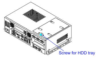
2. Loosen 4 screws, attach your HDD, tighten these screws to fix the HDD and connect the related cables to the motherboard.
