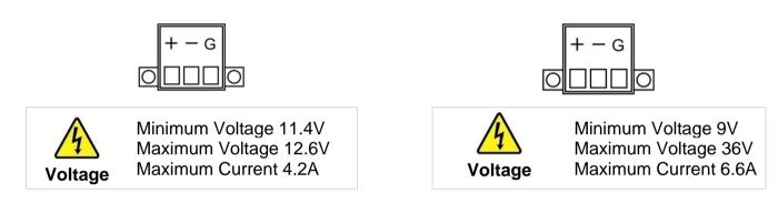
Pin assignment and signal name of the DC power jack connector
