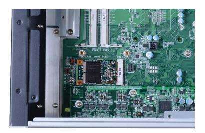
3. Push the mSATA card down until the clips at each end of the latch lock into position. You will hear a distinctive "click", indicating the card is correctly locked into position.
