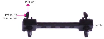
3. Pull the clips up and remove the latch.
