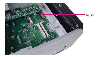
2. Grasping the mSATA card by its edges, align the card into the slot at an approximately 30 degrees angle. Apply firm even pressure to each end of the card until it slips down into the slot. The contact fingers on the edge of the card will almost completely disappear inside the slot.
