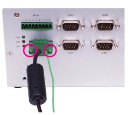
3. Insert one end of the cables into the holes on the terminal block, and use the screwdriver to fasten the cables.
