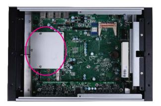
2. The 5 mounting screws on the protective plate is used to secure the plate. Remove these screws and then put them in a safe place for later use.
