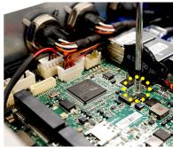
2. Insert the mSATA card into the slot at a 45-degree angle.
