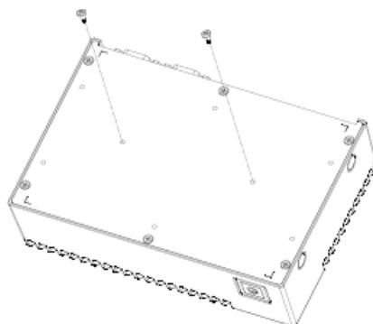
**Step1.** Insert and fasten two M3\*L11.1 screw on the bottom.
