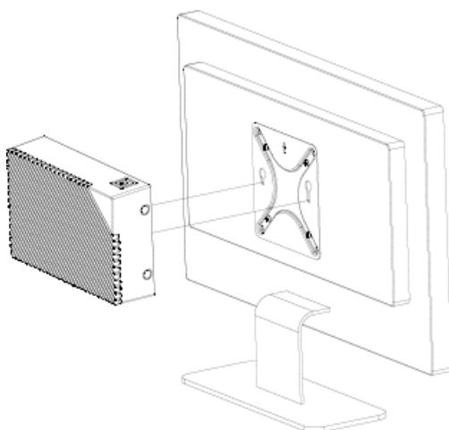
**Step3.** Slide the system onto the VESA mount bracket.
