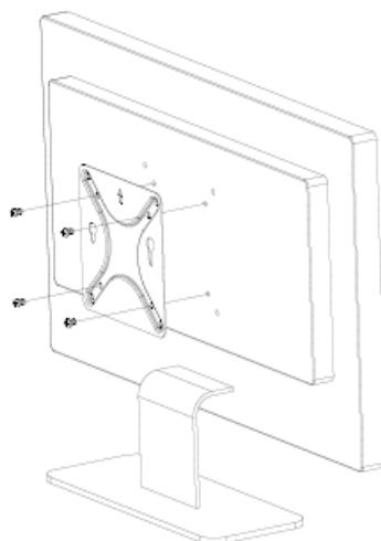
**Step2.** Fix with four M4\*6mm screws on the monitor (or wall).
