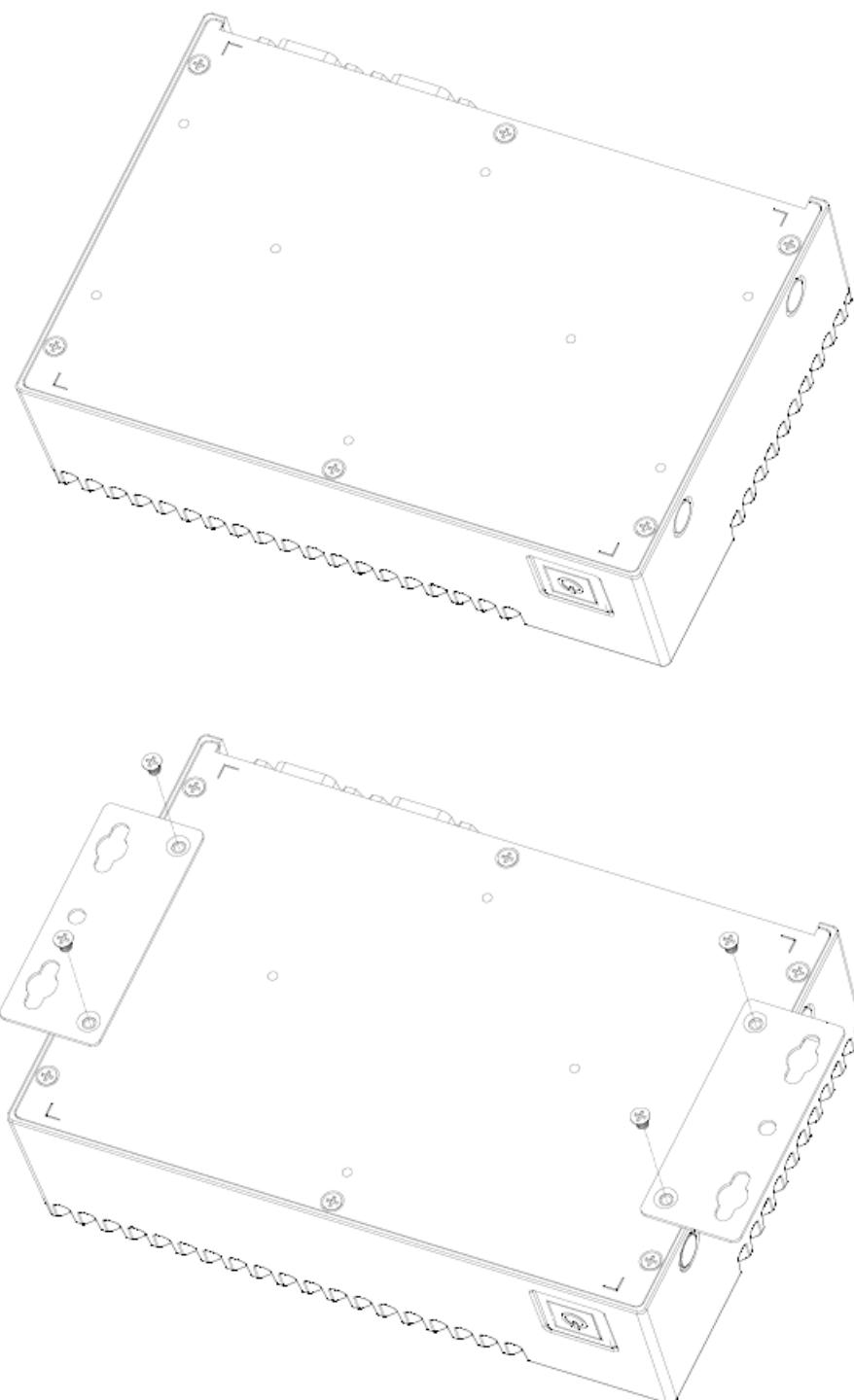
**Step1.** Fasten 4 screws on each side of the system to secure Mounting brackets.
