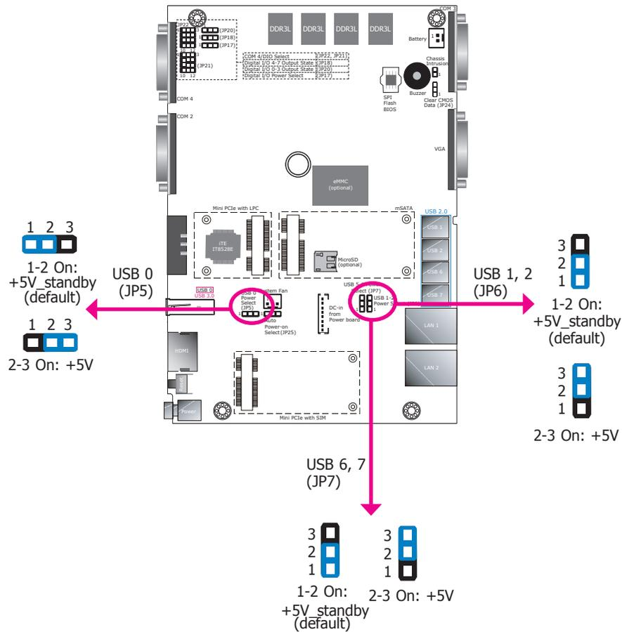
JP5, JP6 and JP7 are used to select the power of the USB ports. Selecting +5V\_standby will allow you to use USB devices to wake up the system.
