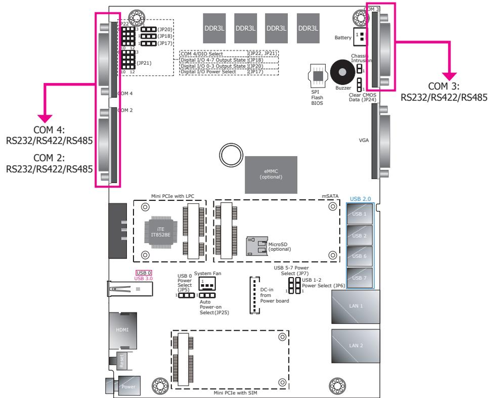
COM 2, COM 3 and COM 4 can be selected among RS232, RS422 and RS485. In addition, COM 4 can be used as a serial, an 8-bit DIO or a CANbus port; refer to Jumper Settings in Chapter 4 for the respective configuration.
