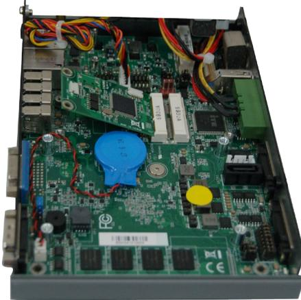
3. Push the Mini PCIe card down and use the provided mounting screws to secure the card on the system board.
