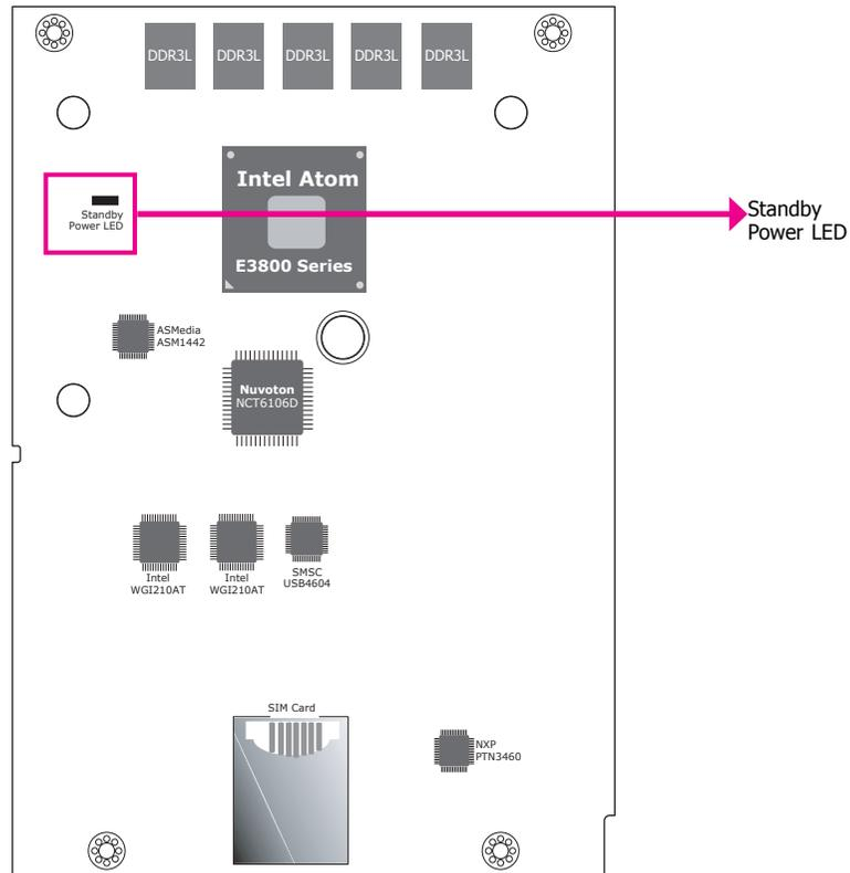
This LED will blink when the system is in the standby mode. It indicates that there is power on the system board. Power-off the PC and then unplug the power cord prior to installing any devices. Failure to do so will cause severe damage to the motherboard and components.
