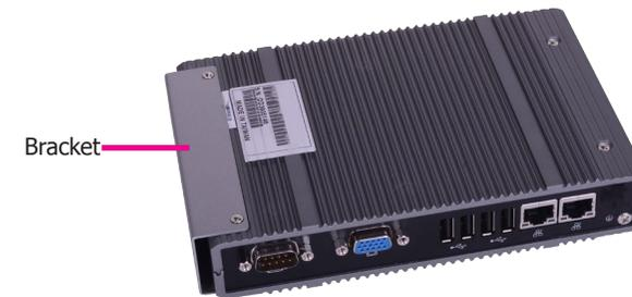
3. Align the mounting holes on the DIN-rail clip with the mounting holes on the bracket, and then use the provided mounting screws to secure the bracket in place.
