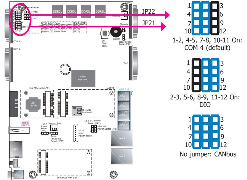
The system board uses JP21 and JP22 to select among serial port COM 4, 8-bit DIO or CANbus on the front panel.
