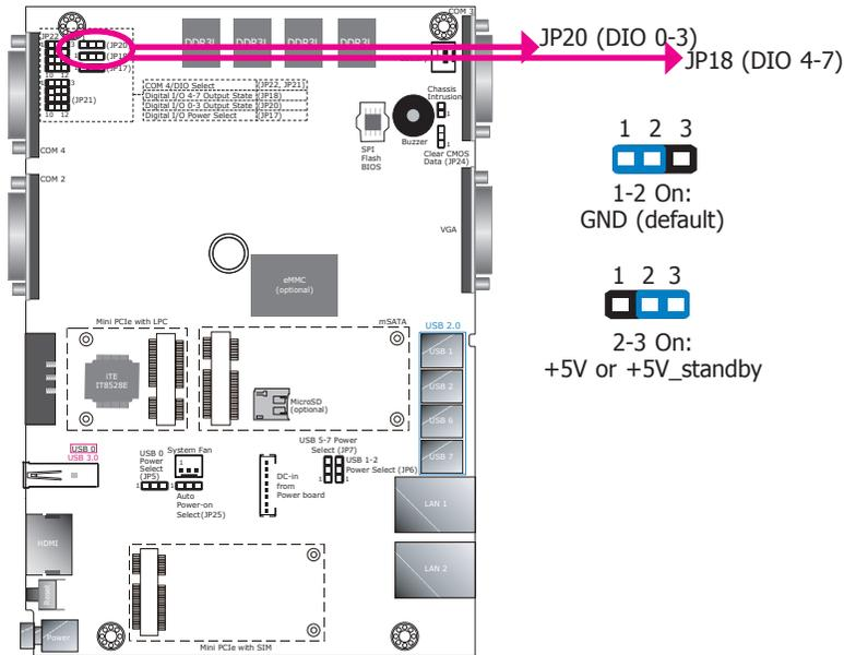
JP20 (DIO pin 0-3) and JP18 (DIO pin 4-7) are used to select the state of DIO output: pull-high or pull-low. When the pull-high state is selected, the level of the DIO signal will be the same as the JP17's setting.
