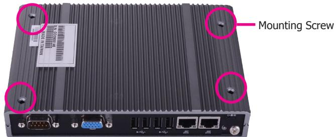
2. At the top side of the system, use the provided mounting screws to secure the wallmount brackets on both sides of the system.
