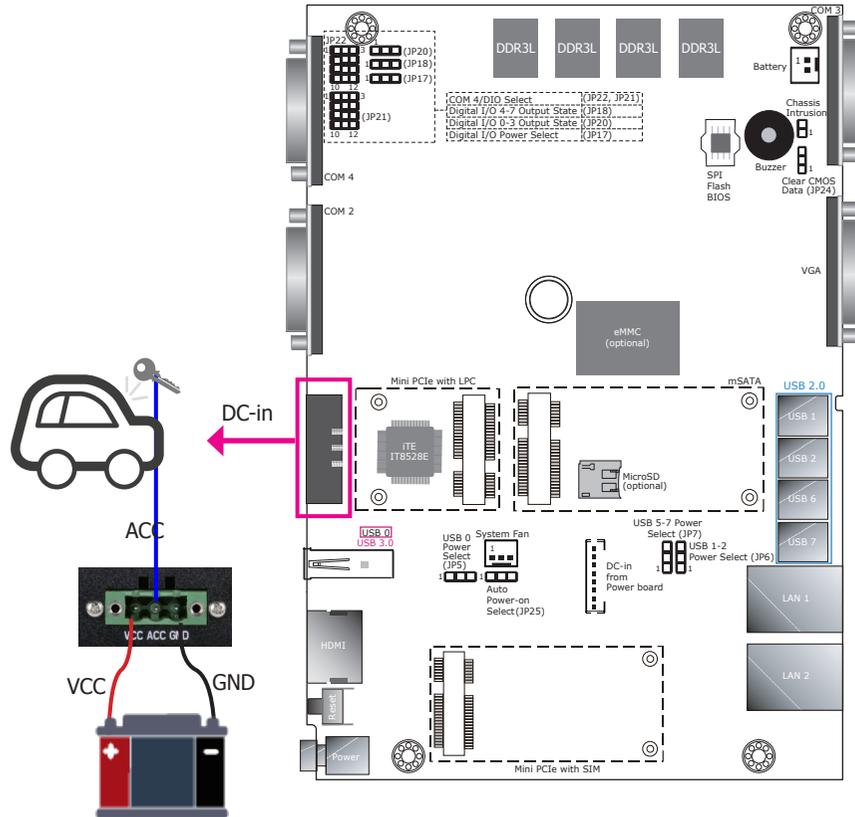
The 3-pole power connector connects to a car battery for power supply. Note that the system accepts a wide power range of 9 to 36V with in-vehicle power management that includes ignition on/off and system on/off delay time control; please refer to the table on the right for more information.
