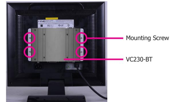
4. The following diagram shows the location and dimension of the VESA-mount screw holes.
