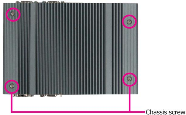
4. After removing the mounting screws, lift the bottom side of the chassis cover to open the system. To access the Mini PCIe and the micro SD slots, remove the four screws to uninstall the power board.
