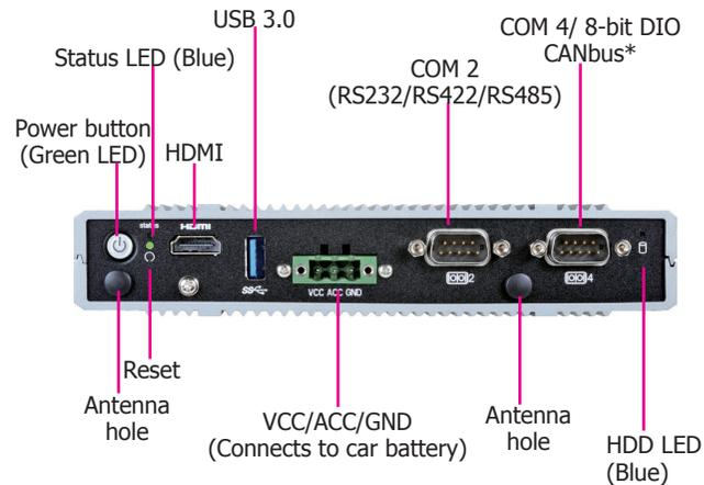
The front panel I/O port consists of the following ports:
