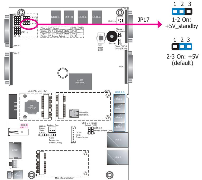
JP17 is used to select the power of the DIO (Digital I/O) signal.
