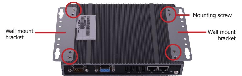
3. The following diagram shows the location and dimension of the wall-mount screw holes.
