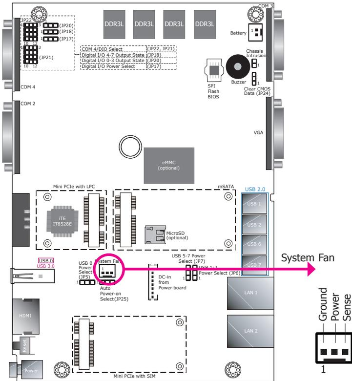
The fan connector is used to connect the cooling fan. The cooling fan will provide adequate airflow throughout the chassis to prevent overheating the CPU and system board components.
