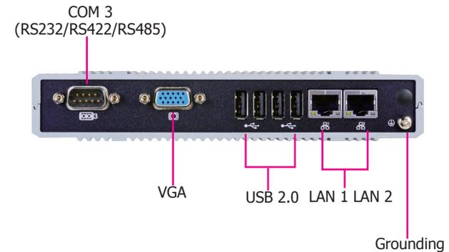
The rear panel I/O port consists of the following ports:
