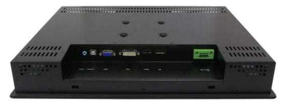
Figure 1.8: Rear View of ADP-1174A
