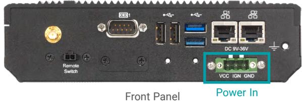
The 9V~36V In box headers are for ignition and power input to the power board, which then converts to 12VDC for output to the system board.
