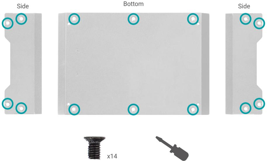
For particular models, there is a memory heatsink attached to the inside of the bottom cover. When installing, orient the bottom cover so that the heatsink sits right on top of the memory.
