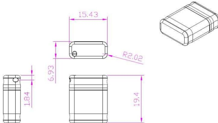
(Tolerance is  $\pm 0.2\text{mm}$ )
