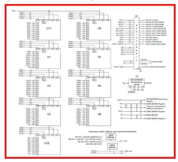
Note: 1. The ZQ ball on each DDR4 component is connected to an external  $240\Omega \pm 1\%$  resistor that is tied to ground. It is used for the calibration of the component's ODT and output driver.
