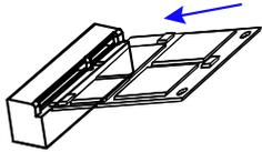
2. Push the mini PCle card downwards as shown in the picture, and fix it with a screw.
