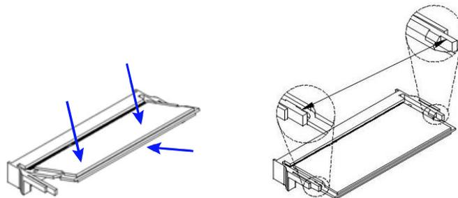
1. Align the key of the memory module with that on the memory slot and insert the module slantwise.
