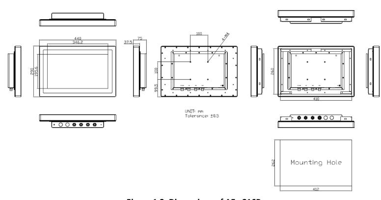
Figure 1.2: Dimensions of AEx-816P
