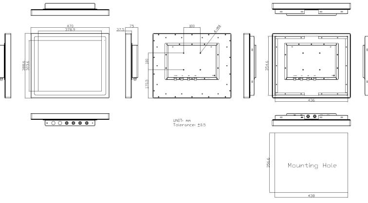
Figure 1.3: Dimensions of AEx-819P(H)
