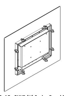
Figure 1.8: AEx-8XXP (H) Series Panel Mounting
