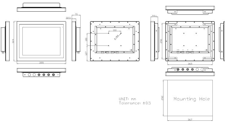
Figure 1.1: Dimensions of AEx-815P(H)
