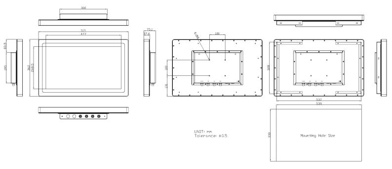
Figure 1.4: Dimensions of AEx-821P
