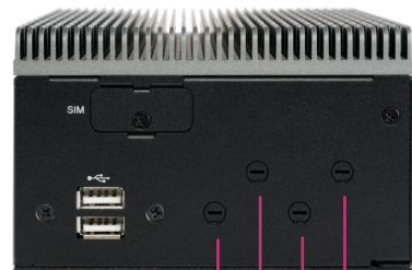
Knockout tabs for antenna holes
