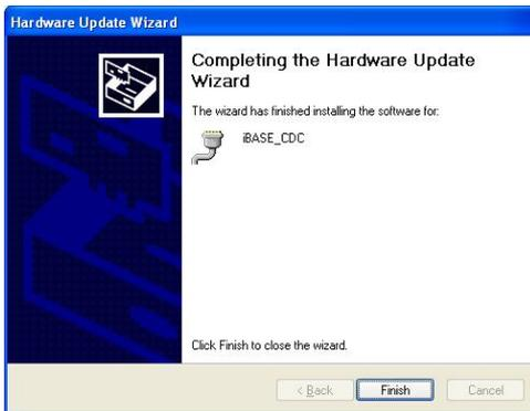
8. There are a total of two serial ports. Therefore, the Hardware Update Wizard procedure has to be repeated for the rest of the serial ports
